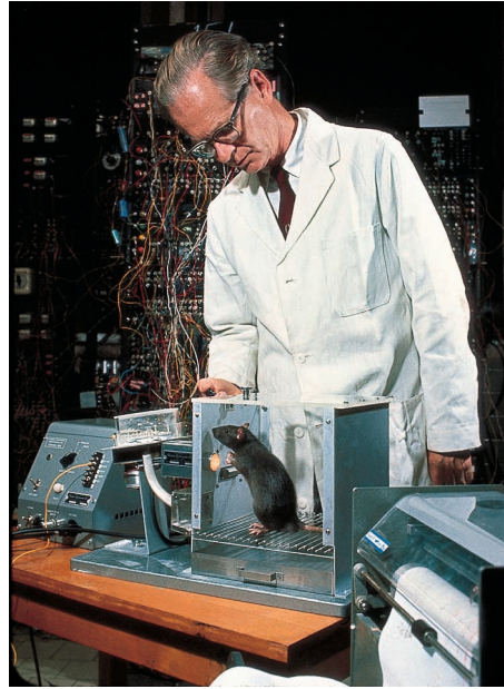
FIGURE 2 B. F. Skinner with a Skinner box used to study operant conditioning. Laboratory rats learn to press the lever in order to obtain food, which is delivered in the tray.
