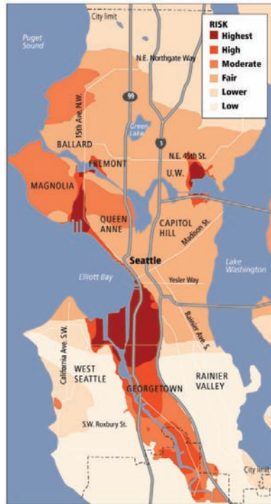
FIGURE 3.9 Seattle Urban Seismic Hazard Map, showing ground motions for the 10 percent chance of exceedance in 50 years or a 1 percent chance of exceedance in 475 years. SOURCE: Hearst Corporation. Available at seattlepi.com/U.S.G.S .
