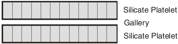
Fig. 1 Idealized layered silicate structure
