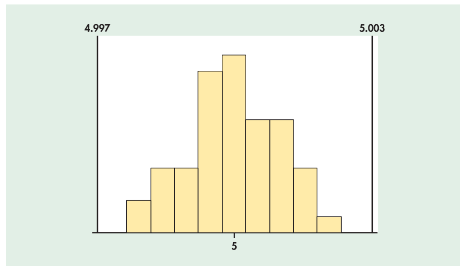
FIGURE 13.1 Histogram of a sample of the dimensions (millimeters) of 50 manufactured parts, with the tolerance limits indicated.
