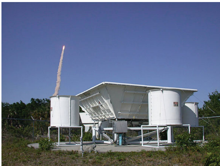
Fig. II.9.5 NOAA developed and Radian fielded boundary layer wind profiler at Cape Canaveral FL during the launch of the Space Shuttle
