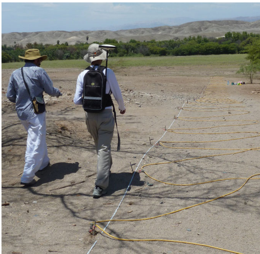
Fig. 23.3 GNSS kinematic survey along a geoelectrical line in Cahuachi
