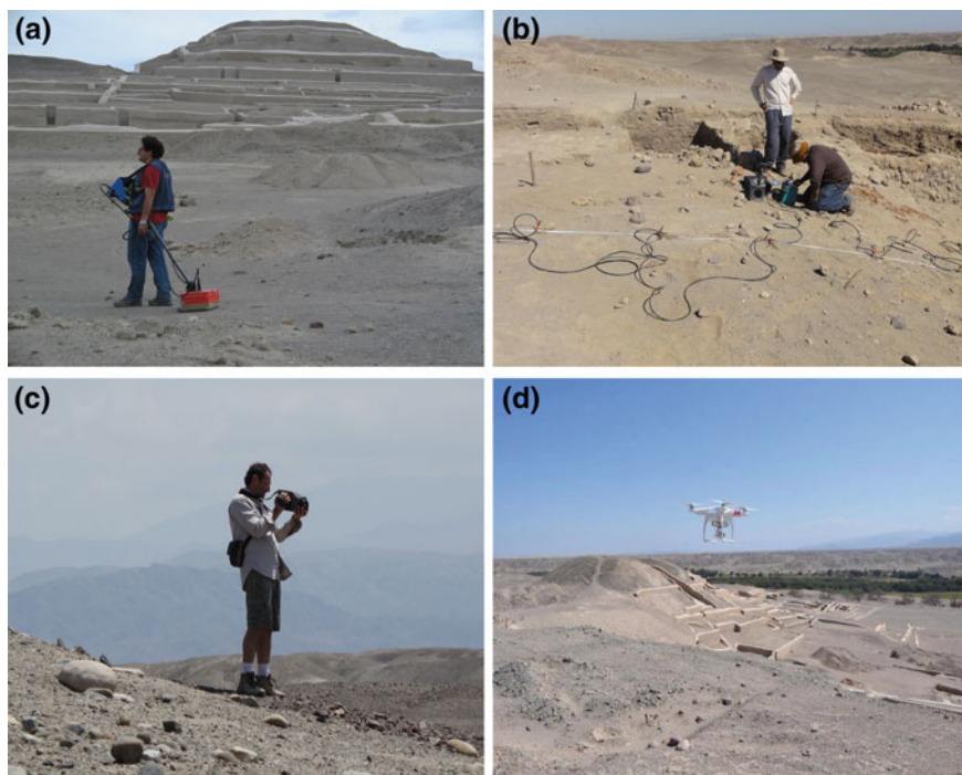
Fig. 1.14 Various methods and techniques used for investigating and mapping buried and shallow archaeological remains in Cahuachi and in Nasca territory, such as a georadar, b electrical resistivity tomography, c magnetometry, infrared thermography, and d aerial prospection by ultra-light aircrafts and UAVs
