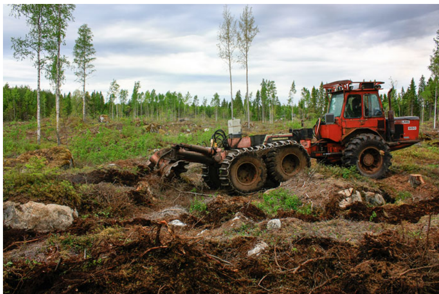
Fig. 5.2 Soil preparation in progress. Large blades break the surface ground exposing mineral soil where new trees will be planted (photo by Piritta Häkälä/SKAIK, Finnish National Board of Antiquities)
