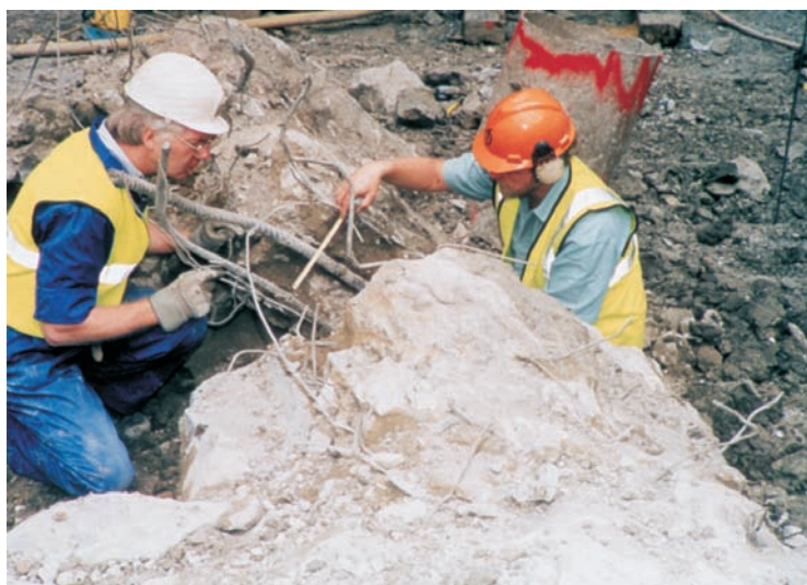
Figure 14.6 Example of logging concrete in the field requiring examination of different types of concrete and reinforcements.
