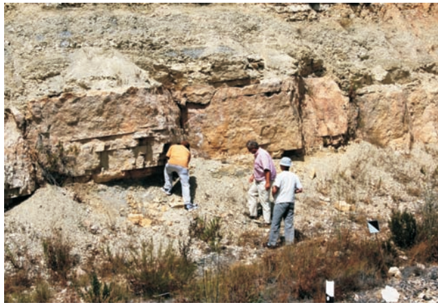
Figure 2.2 Interbedded sandstones and mudstones in Spain undergoing weathering as envisaged by the column 3 approach in Table 2.5 (photograph courtesy of Steve Hencher).
