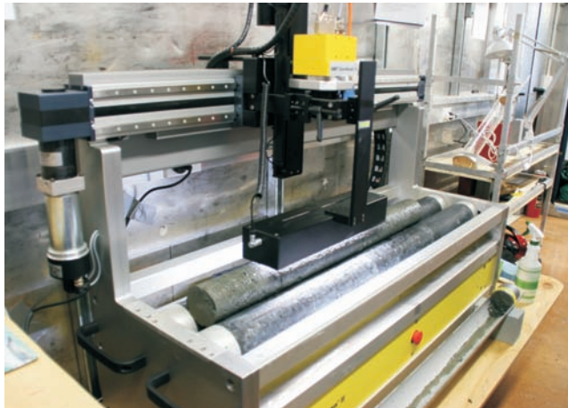
Figure 16.9 Core scanner for high resolution imaging of cores, around whole circumference if core is sufficiently intact (photograph courtesy of DMT GmbH & Co. KG).
