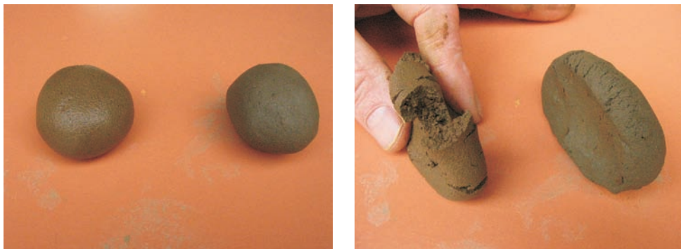
Figure 4.16 Cohesion of fine soils. The silt on the left breaks and starts to crumble, whereas the clay on the right deforms without rupture.
