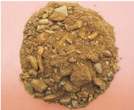
Figure 4.7 Mixture of sand and gravel with a number of particles around the 2 mm size, which many loggers describe incorrectly.
