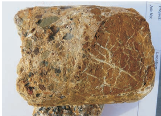
Figure 4.20 Metasomatically altered brown harzburgite cobble within caliche (carbonate cemented gravel) containing chert and green gabbro fragments; this could be described as ‘conglomeratic LIMESTONE’; core diameter is 80 mm (photograph courtesy of Steve Macklin).
