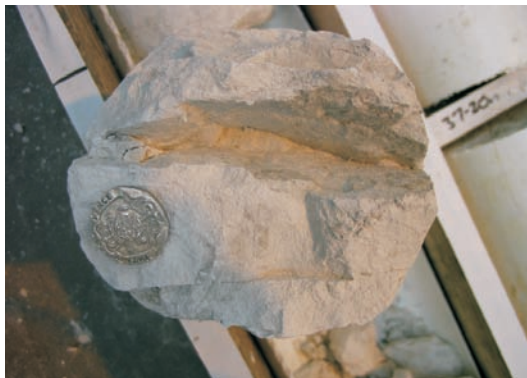
Figure 11.3 Chalk core containing at least three vertical discontinuities, allowing the spacing to be described, even though this may still not be representative as the sampling of axis parallel fractures is not usually complete.
