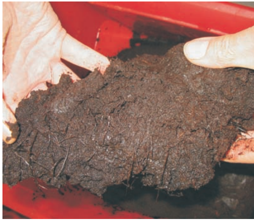
Figure 13.2 Typical peat showing both decomposed material and fibres.
