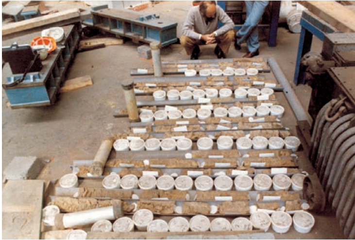
Figure 16.2 Laying out all the samples before starting the logging of a borehole (photograph courtesy of Soil Mechanics).
