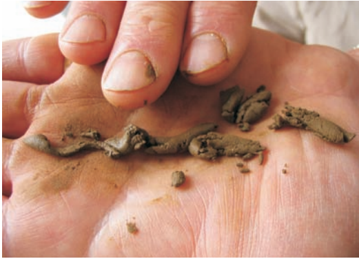
Figure 4.12 Carrying out the toughness and plasticity hand tests by rolling and rerolling the soil to form 3 mm threads.
