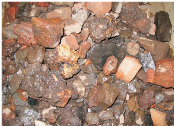
Figure 14.2 General fill comprising processed gravels as well as bricks and burnt shales.
