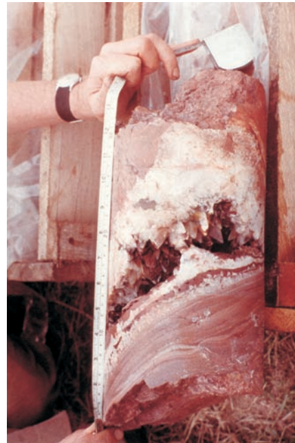
Figure 8.8 Example of other information in the form of voids in the core.
