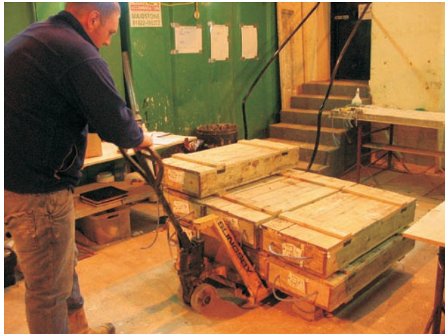
Figure 1.7 Use of appropriate handling equipment in and around core and sample stores areas can reduce the risk of manual handling incidents and injury to loggers.
