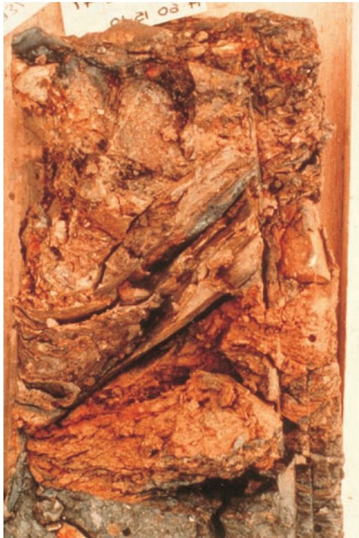
Figure 14.1 Embankment fill showing clods of different coloured clays (and a throughgoing shear surface).
