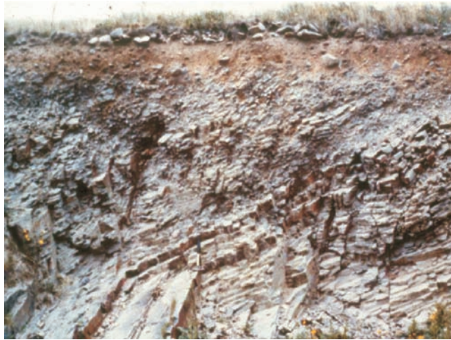
Figure 1.6 Exposure of gradational rockhead passing from bedrock at the base of the cliff to transported soil at the top. Various different rockhead levels could be defined within this gradation.
