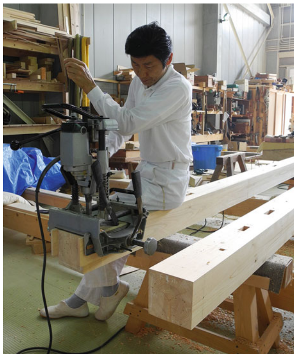
Fig. 13 Yamada Workshop—power tools. Power tools are in frequent use. Holes for the tenons are made with a portable mortiser, an overhead router is used for plugs. Photo by Christoph Henrichsen, May 2011
