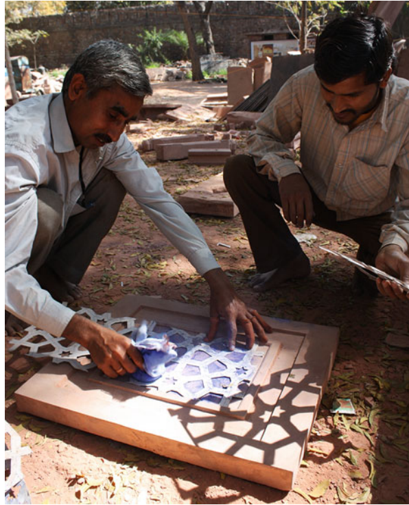
Fig. 6 Demonstration of the transference of a geometric pattern onto sandstone with the help of a template and blue powder. Photo by Katharina Weiler, March 2010
