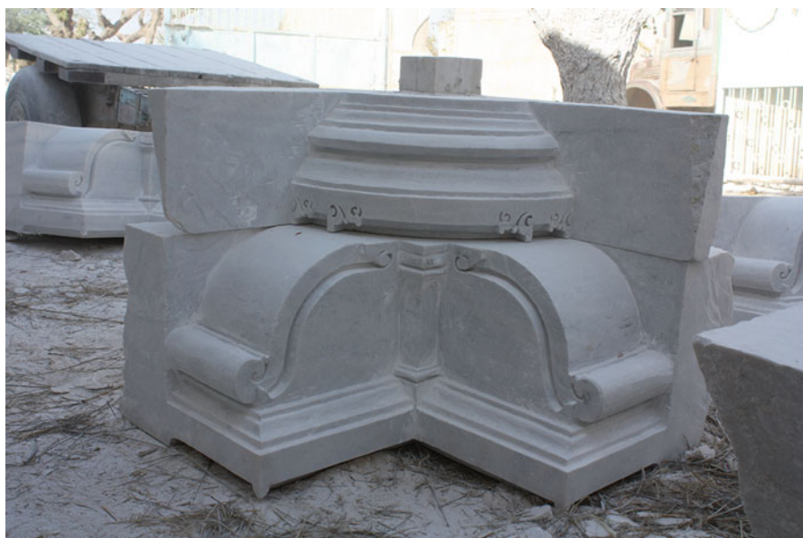
Fig. 20 Makrana: The inverted capital and torc of a pillar for Shri Jain Vardhaman Tirthah taking shape. Photo by Katharina Weiler, March 2010
