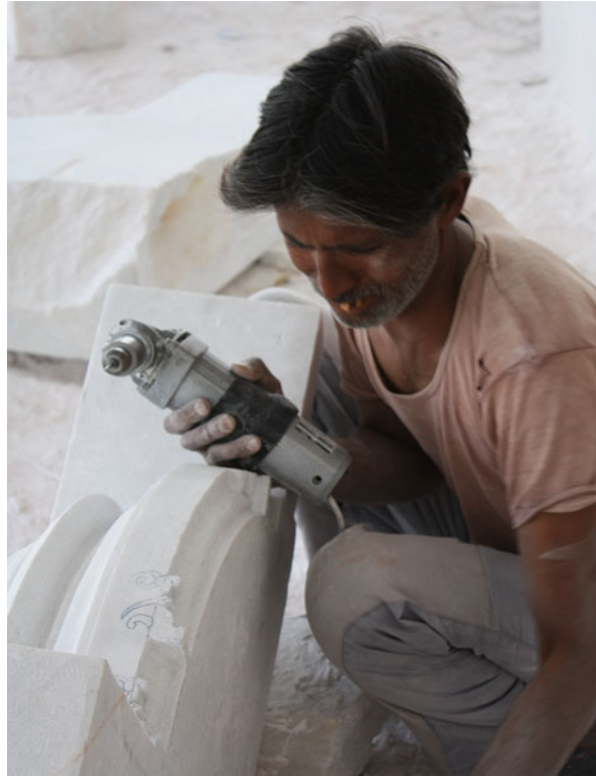
Fig. 19 Makrana: Electric tools are used in the process of fine carving following the imprints on the marble torso of a pillar for Shri Jain Vardhaman Tirthah. Photo by Katharina Weiler, March 2010
