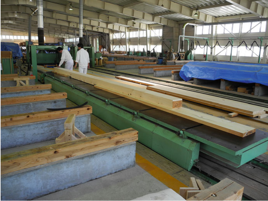
Fig. 12 Yamada Workshop—Machine hall. View of new machine hall in the Yamada workshop. The amount of machine work has increased considerably. Members of the frame are worked to the desired dimensions with large planers and thicknessers. Photo by Christoph Henrichsen, May 2011
