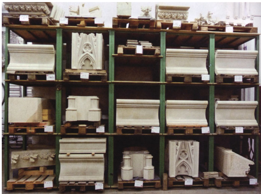
Fig. 43 Cologne Cathedral. Cornice moldings, facing tracery, and fragments of pinnacles, newly crafted to replace weather-damaged elements on the southern transept, spring 2008. Source: Schock-Werner 2008, 260
