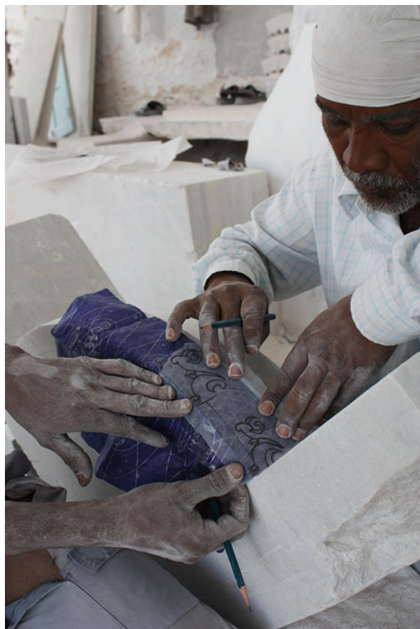
Fig. 18 Makrana: Craftsmen provided with the measurements and different patterns for the torc of a pillar for the Shri Jain Vardhaman Tirthah. The pattern is printed on tracing paper, scale 1:1. The craftsmen copy the pattern with the help of carbon paper that imprints each design on the surface of the marble. Photo by Katharina Weiler, March 2010
