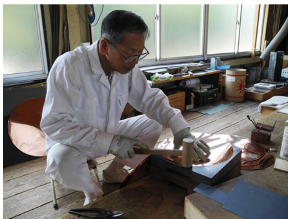
Fig. 14 Yamada Workshop—copper sheet for posts. The feet of the posts are clad with thin copper sheeting to reduce rotting. Photo by Christoph Henrichsen, May 2011
