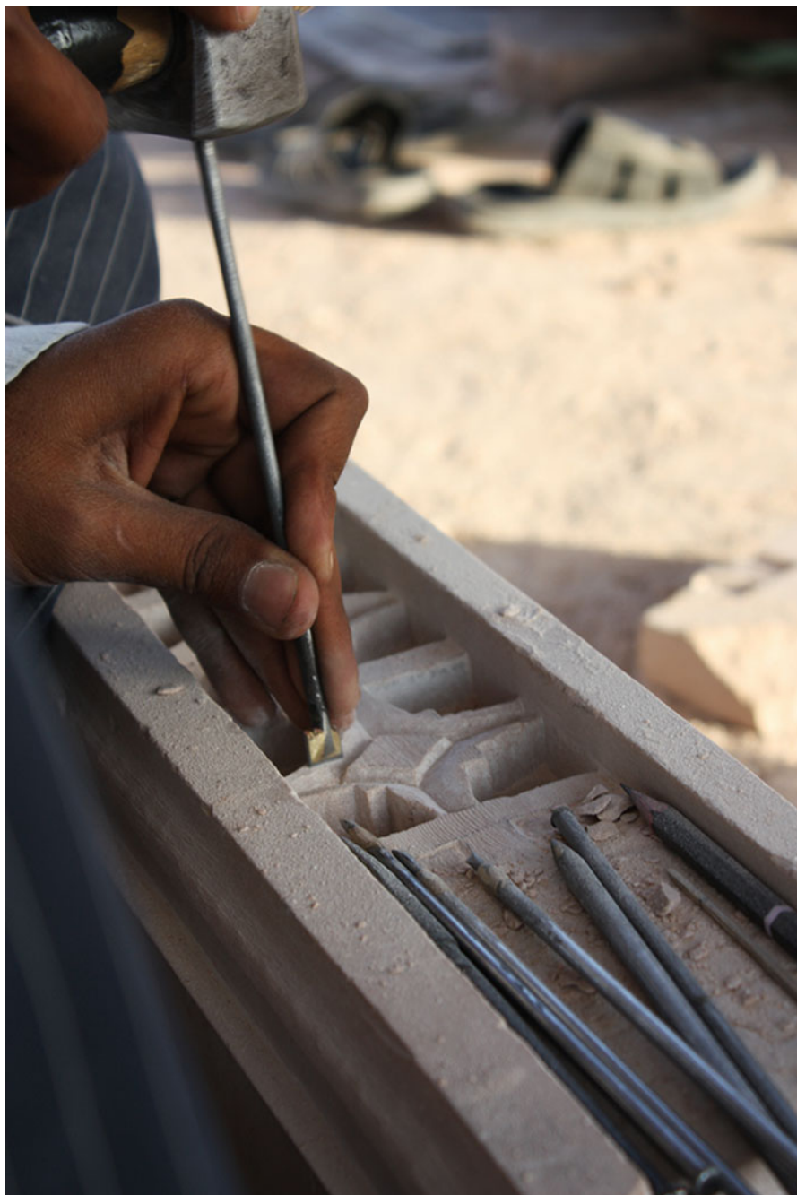
Fig. 10 Using different chisels, a sculptor brings out the floral design of the bas relief. Photo by Katharina Weiler, March 2010
