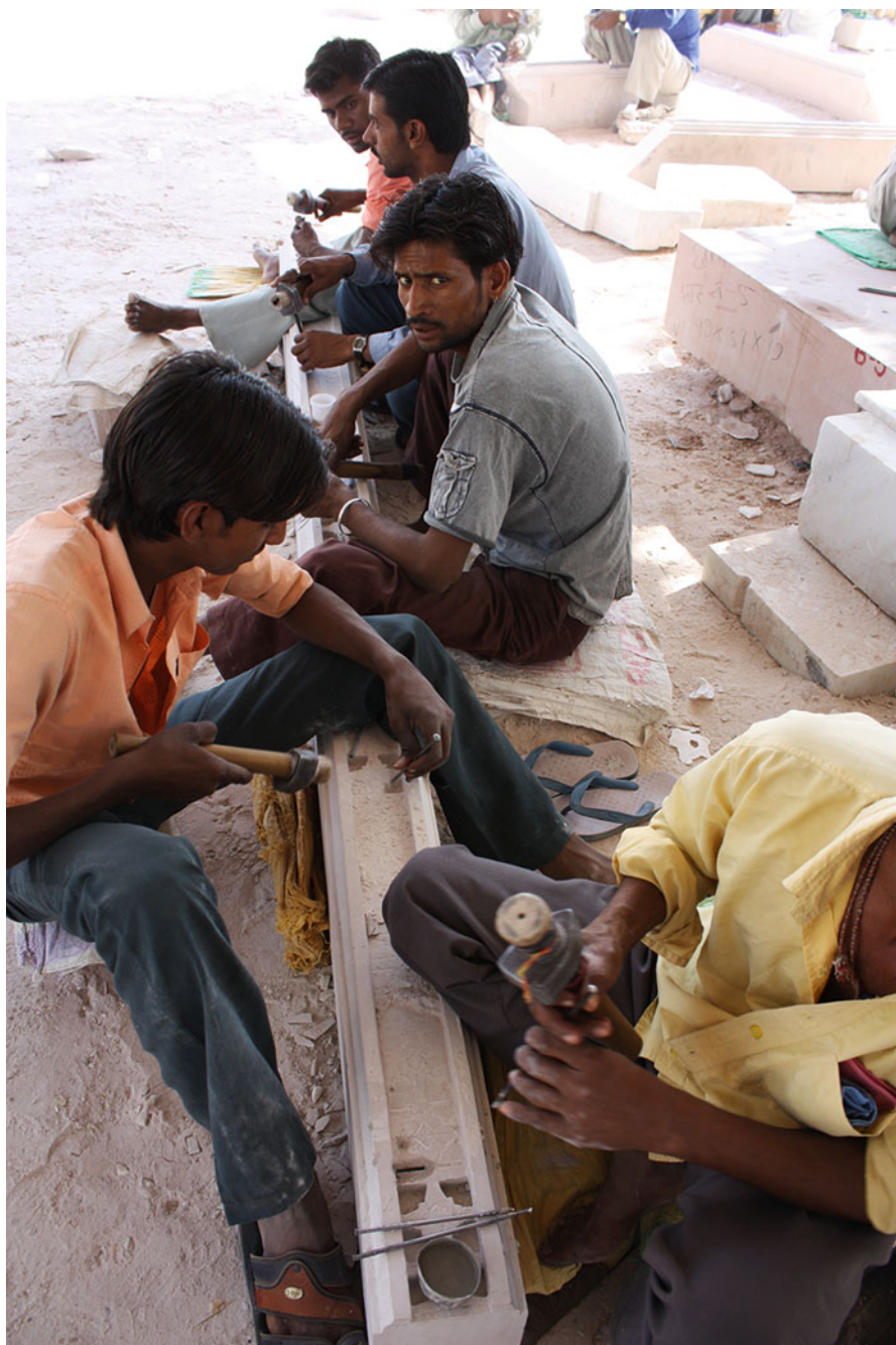
Fig. 9 Up to five men work on a single block of sandstone. Each worker carves the same décor while shaping the stone with his tools. This kind of teamwork takes account of the fact that people work at different speeds. At any one time the sculptors will have arrived at different stages in their carving work. Photo by Katharina Weiler, March 2010
