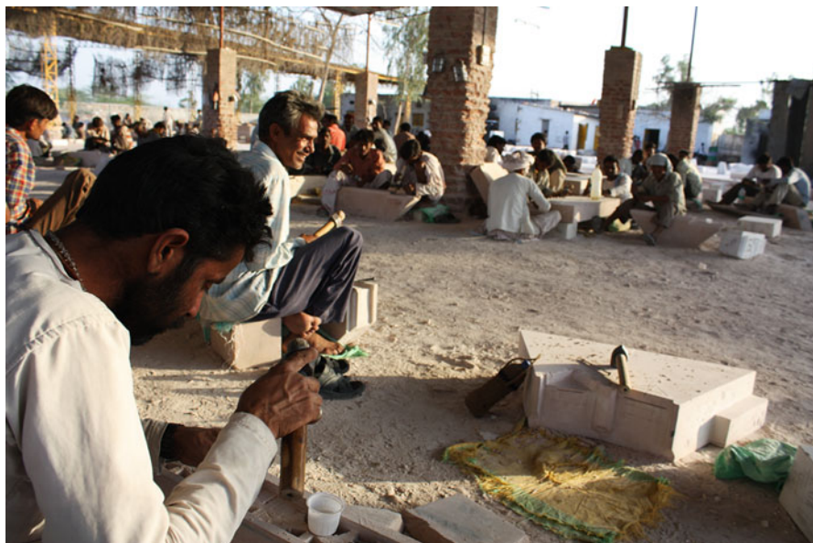
Fig. 7 Siwera: The craftsmen work singly or in groups, formed in accordance with the different types of building elements or layers they are manufacturing, e.g., plinth, beams, pillars, or ceiling. Photo by Katharina Weiler, March 2010
