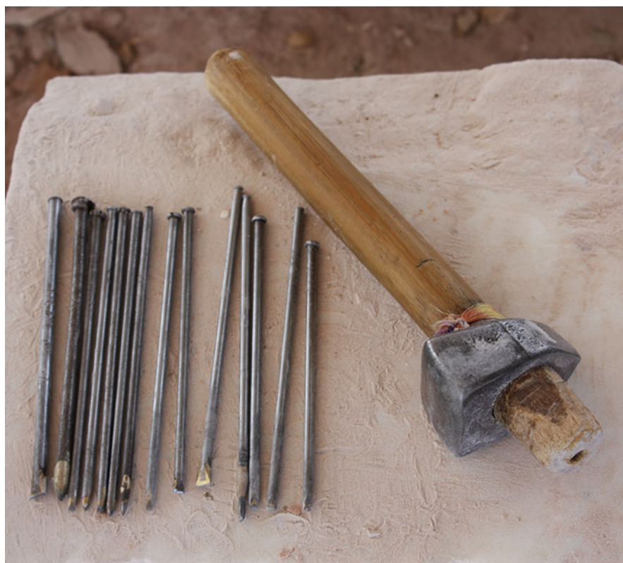
Fig. 8 Tools: A hammer with a hollow shaft for blowing away stone dust and a range of 14 different carving chisels. Photo by Katharina Weiler, March 2010
