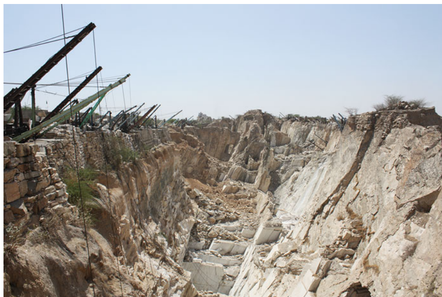
Fig. 14 Makrana, Rajasthan: The Sahib wali quarry houses a dozen mines, separated by high marble walls. Cranes look down on the mines, their ropes extending into the depths. The marble is mined from a current depth of more than 100 m. Photo by Katharina Weiler, March 2010
