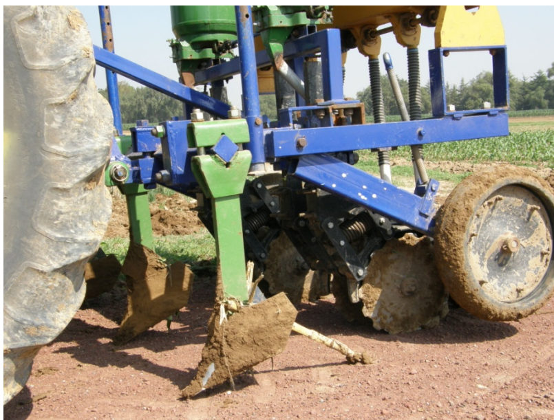
Fig. 5. Prototype of disk-type planter for small-grain cereals and maize developed for the planting system on permanent beds.
