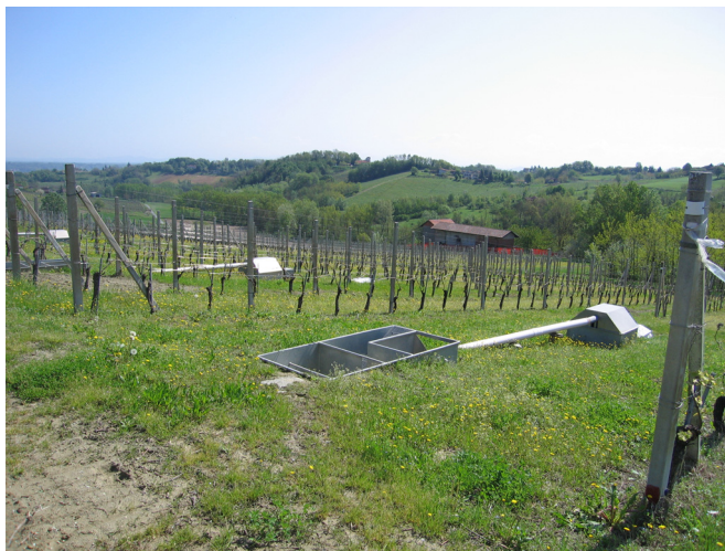
Fig. 7. Sedimentation trap and tipping-bucket device for runoff discharge measurements.
