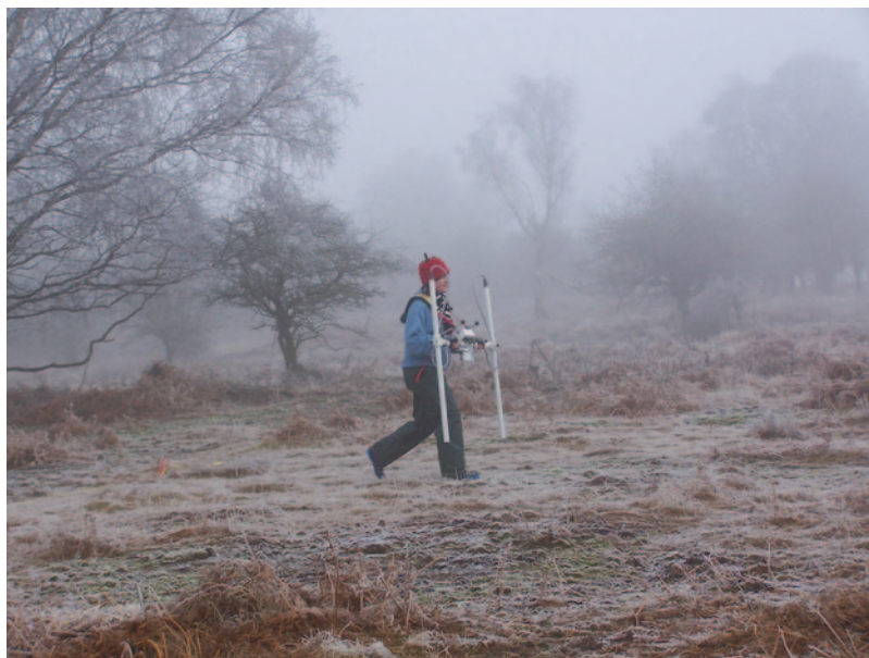
Fig. 7.5 Magnetometry survey being carried out using a fluxgate gradiometer. (Copyright: Caroline Sturdy Colls)
