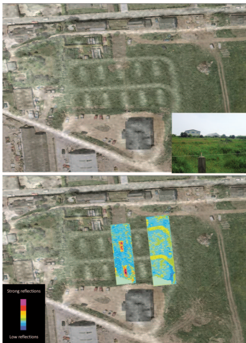
Fig. 5.12 A historic aerial image of a potential labour camp on the island of Alderney overlaid onto a modern aerial image ( top ). The structures visible in the image were no longer visible on the surface ( top inset ) and they were located using Ground Penetrating Radar (GPR). (Copyright: Caroline Sturdy Colls/Google)
