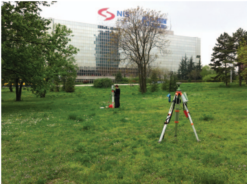
Fig. 6.13 A differential kinematic GPS system (foreground) and total station (background) being used to collect topographic survey data at the former Semlin camp in Serbia. (Copyright: Caroline Sturdy Colls)
