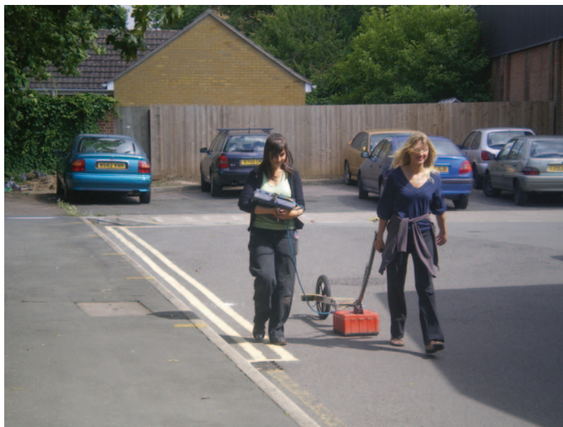
Fig. 7.1 Conducting a GPR survey over a Jewish cemetery that was believed to exist beneath a modern road and car park. (Copyright: Caroline Sturdy Colls)
