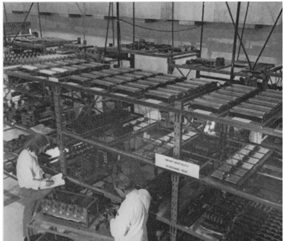
Fig. 8.2. This is a view of a rig which is testing heater elements (top shelf) and their control units (second shelf): for infant mortality type failure during functional operation
