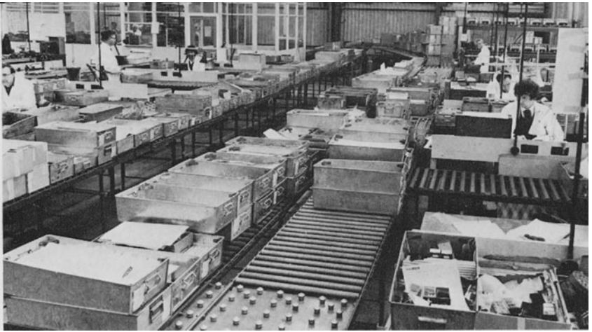
Fig. 5.1. This shows a goods inwards inspection area laid out on the roller-track principle
