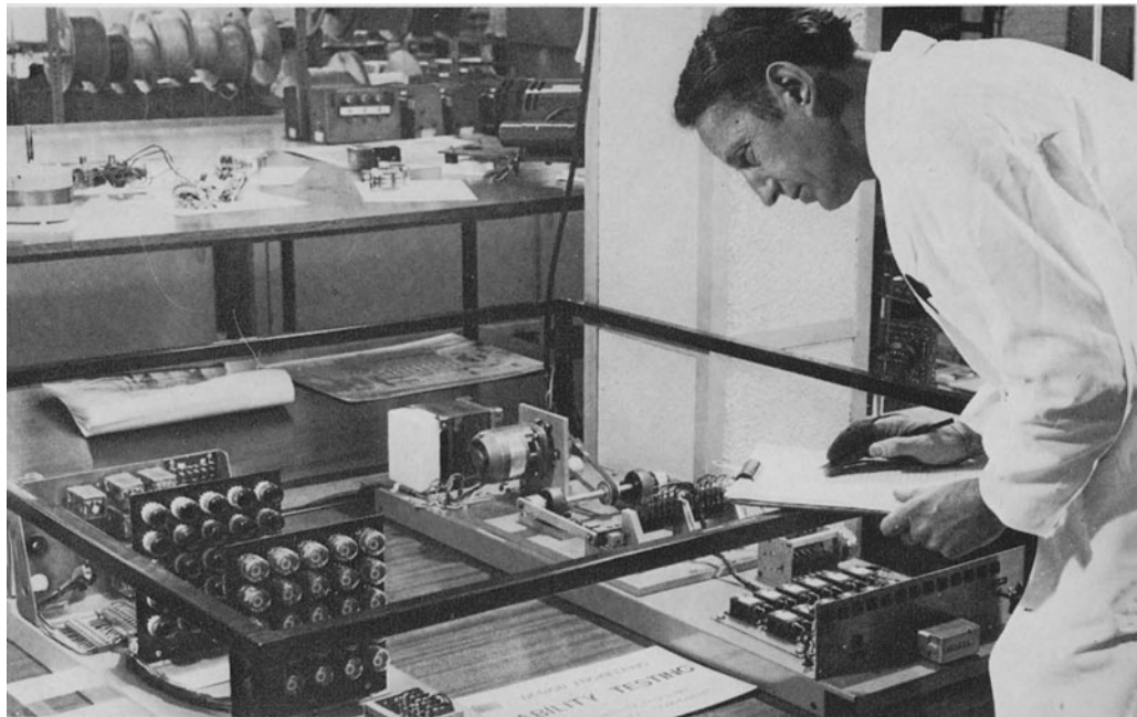
Fig. 8.4. On the left is a rig for testing number indicator tubes commonly known as 'Nixies'. In the view, the number 6 is illuminated on the front bank of tubes. On the right the rig is for testing microswitches. A bank of switches under test is visible just below the clip of the test engineer's clipboard
