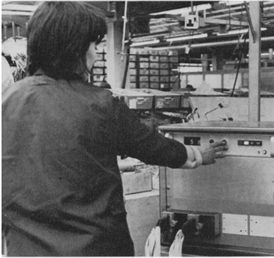
Fig. 7.3. An automatic control system for the electrical sub-assemblies produced on the wiring jig in Fig. 7.2
