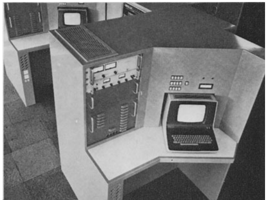
Right Fig. 5.4. A modern quality control device using computer technology for testing electric and electronic components
