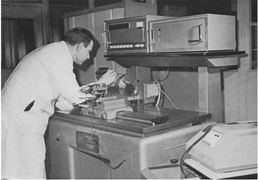
Fig. 3.6. Automatic Cam Profile Test equipment with a punched tape reader (right) controlling the angular dividing head, linear displacements of which are measured and recorded
