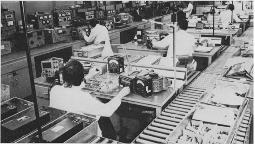
Fig. 5.2. An electrical test section laid out on the roller-track flow system
