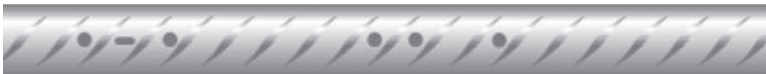
Figure 12.1 CARES bar marks. The dot-dash-dot (shown on the left) is the CARES registered certification mark (number 2150684) and indicates that the product is CARES approved. The number of ribs between the next two dots after the CARES approval mark, indicate the country of origin. The number of ribs between the next two dots indicates the steel mill number. Details of steel mill numbers can be found in either the CARES certificate or the list of 'Firms Holding CARES Certificates of Approval'. Further details or confirmation of barmarks can be obtained from the CARES office. (Courtesy UK Certification Authority for Reinforcing Steels).
