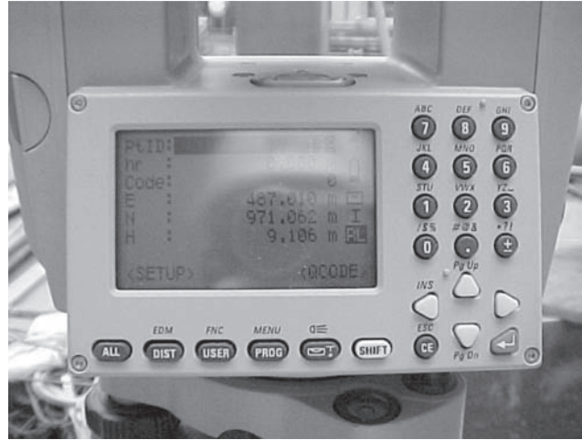
Figure 4.7b Leica Total Station keyboard and display. The display can be changed to show a variety of information i.e. angles and distances. Other makes are similar.
