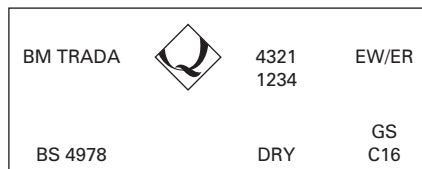
Figure 15.3 Example of a visual strength grading mark.
