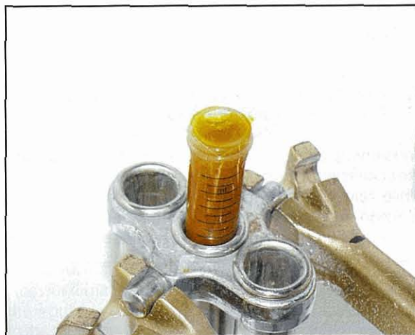
16.3 Centrifuge with free swinging buckets showing a coverslip in place before centrifugation.
