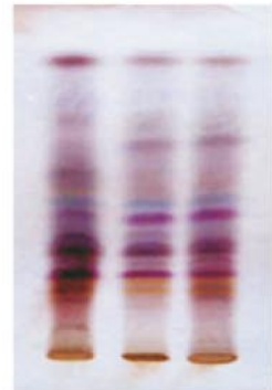
Fig. 19.3 a TLC fingerprint profiles of Chandraprabhavati, a polyherbal formulation [46]. Track 1 : authentic sample; Tracks 2 and 3 : market samples b see next page
