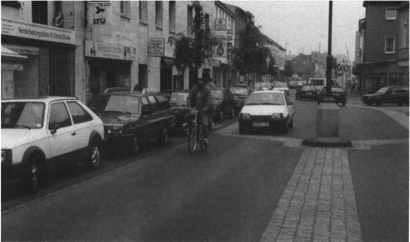
Figure 58. Town centre road space reconstructed to prevent passing manoeuvres – the cyclist as dynamic traffic calming, Hennef, Germany.
