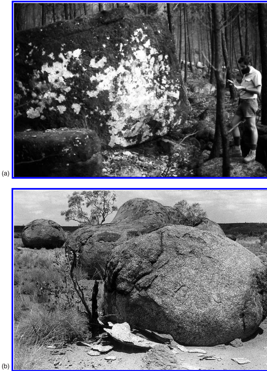
Figure 3.1. Spalling of granite due to bush fires (a) near the Portugal-Galicia frontier line of Portela d'Home; (b) at the Devil's Marbles, Northern Territory. Most fire-induced heating produces thin flakes and slivers, only 2–3mm thick, but here the plates spalled off are several centimetres in thickness.
