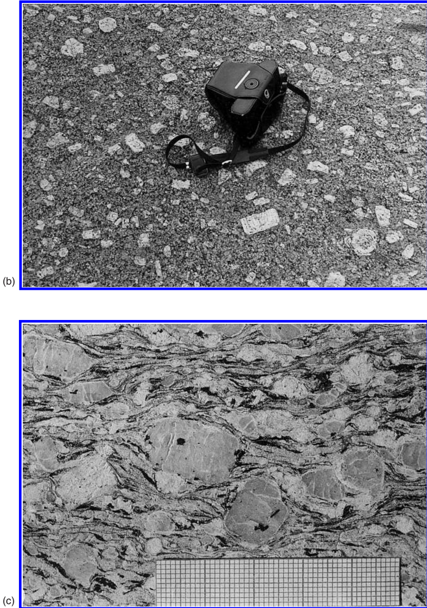
Figure 1.6. (b) Porphyritic granite, South East district of South Australia. (c) Thin section of gneissic granite with augen (“eyes”) of potash feldspar and plagioclase set in layered matrix of biotite and quartz; scale in mm.
