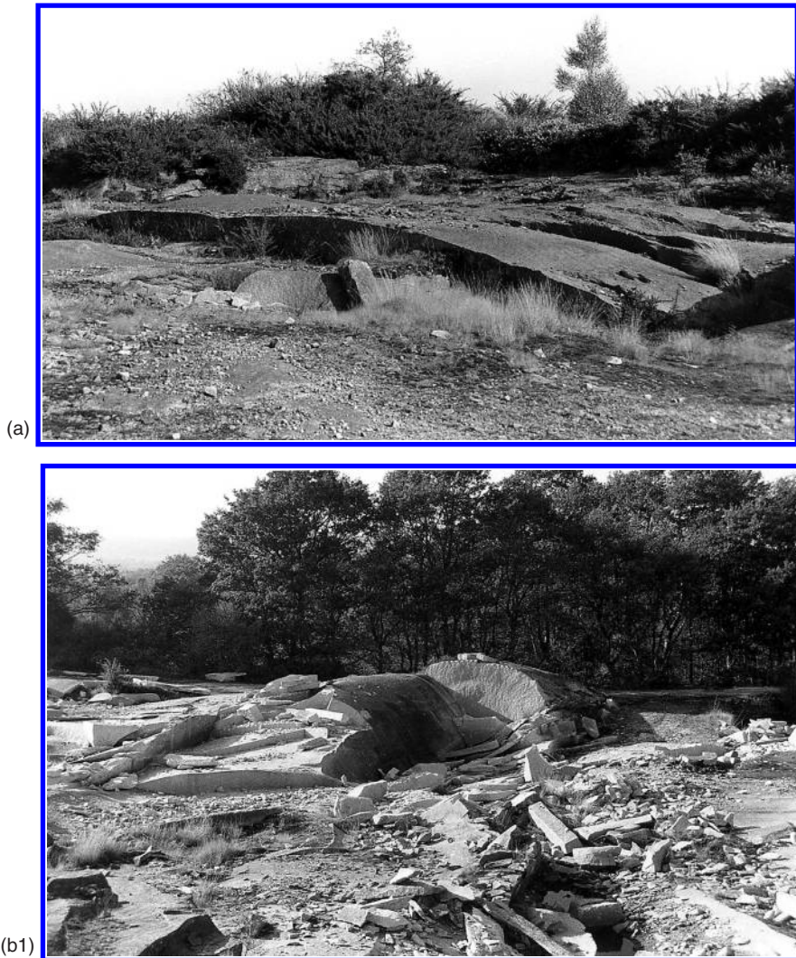
Figure 2.9. (a) Sheet structures. (b1 and b2) Wedge in granite at Mariz Quarry, Guitiriz, Galicia.
