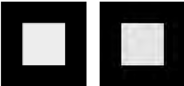
Figure 3.48. JPEG (left) and wavelet (right) compressed square
