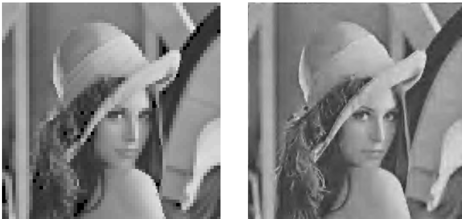
Figure 3.46. Comparison of JPEG and wavelet compression
