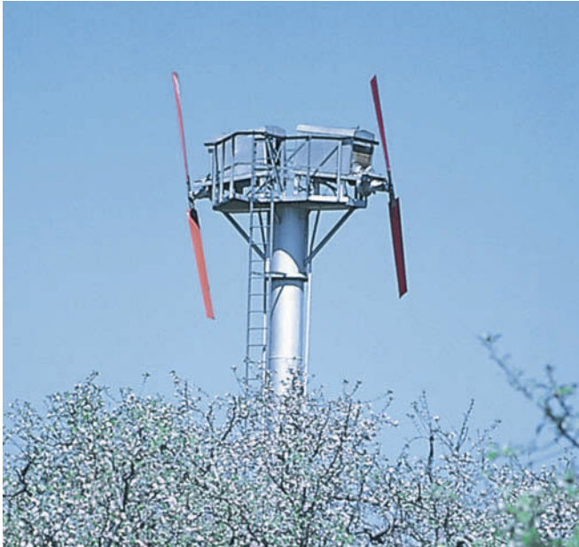
FIGURE 3.7 Wind machines mix cooler surface air with warmer air above.
