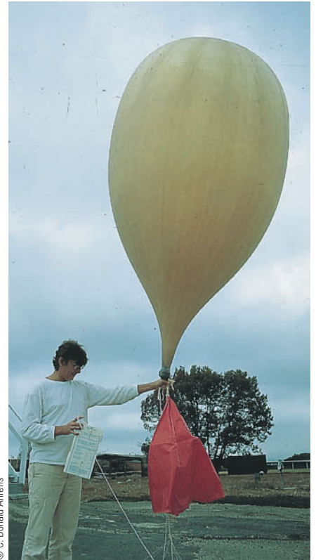
FIGURE 1 The radiosonde with parachute and balloon.
