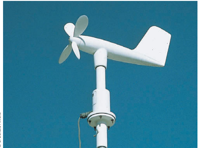
■ FIGURE 6.28 The aerovane (skyvane).
