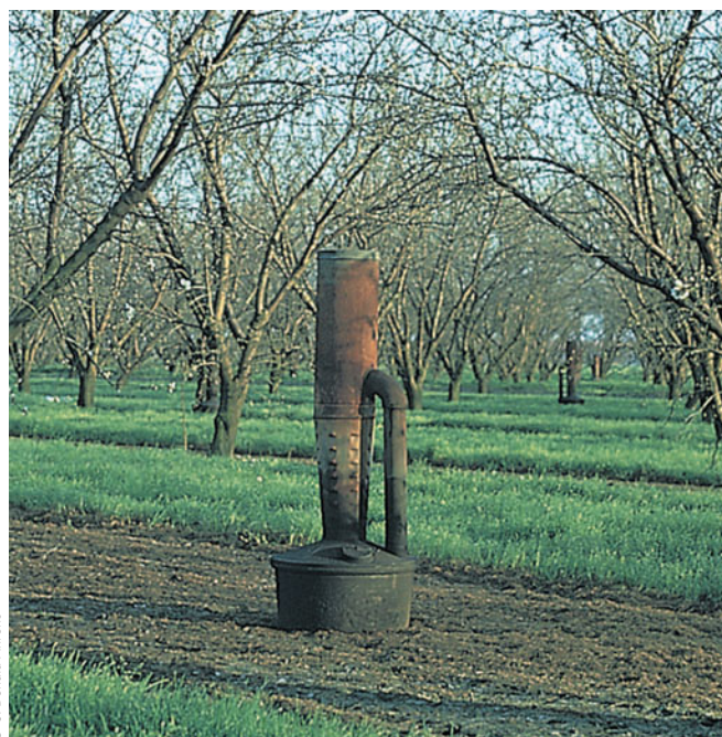
FIGURE 3.6 Orchard heaters circulate the air by setting up convection currents.
