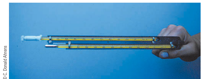
FIGURE 4.11 The sling psychrometer.
