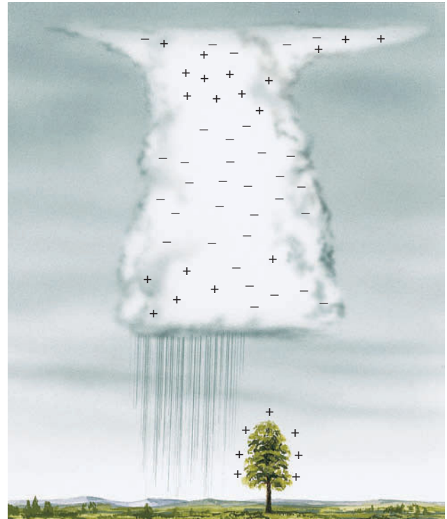
■ FIGURE 10.21 The generalized charge distribution in a mature thunderstorm.
