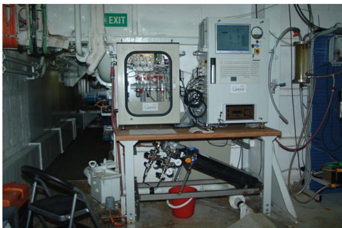
**Fig. 4.3** Automated measurement system on VOS “Finnmaid” for the recording of the surface water pCO<sub>2</sub>
