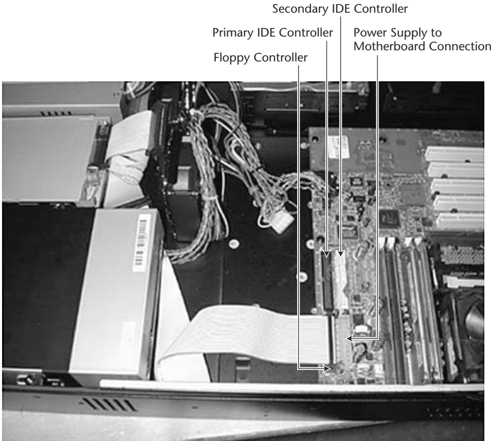
Figure 8.8 Connecting the floppy drive ribbon cables.
