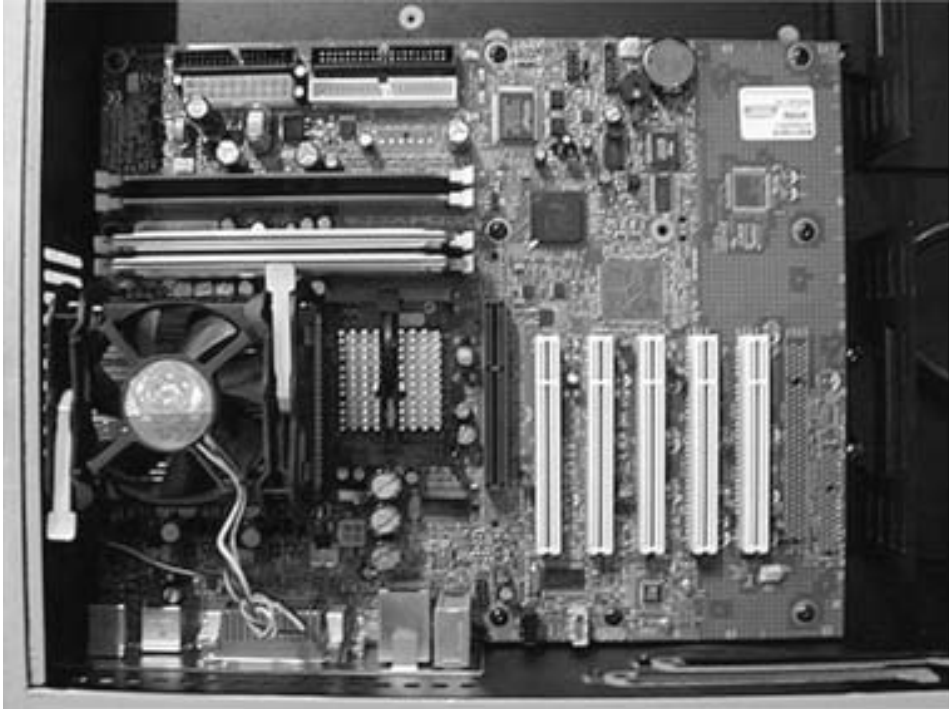
Figure 8.4 Rambus memory in slots 1 and 2, with Crimms inserted in slots 3 and 4.
