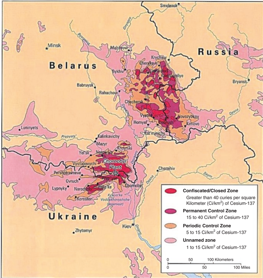
Fig. 2.19 Radiation hot spots over Ukraine and Belarus in the wake of the Chernobyl nuclear accident (137-Cs in Curies/km 2 ). (1 curie = 37.109 Becquerel) ( https://upload.wikimedia.org/wikipedia/commons/2/23/Chernobyl_radiation_map_1996.svg )
