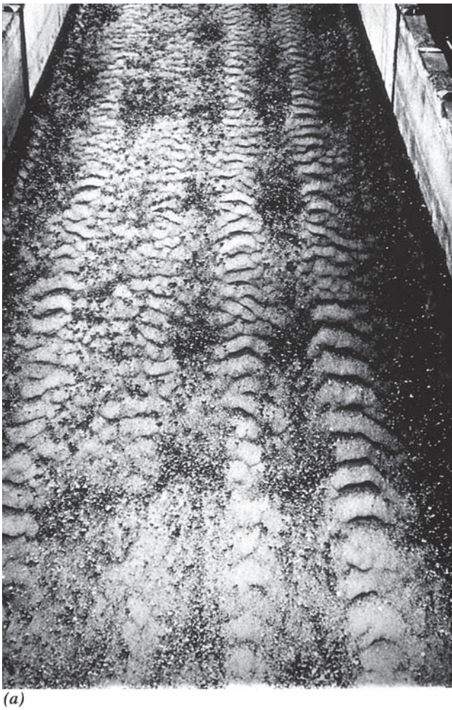
Fig. 3-8. Streaks of sorted sediment in (a) a laboratory flume (from Günter, 1971; courtesy A. Günter) and (b) a river (image courtesy T. Tsujimoto).
