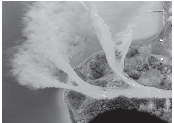
Fig. 1-17. High sediment concentration turbidity currents from Frosst Creek, British Columbia, Canada, plunging through delta into Cultus Lake. Photograph by V. J. Galay.
