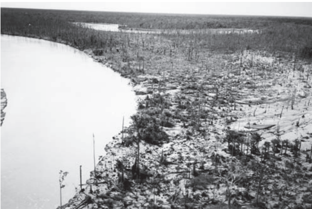
Fig. 1-16. Fly River in Papua New Guinea: an example of man-induced ecological disaster. Sediment deposition from the Ok Tedi mine continues to aggrade riverbeds and amplifies flooding and sedimentation of forest areas, killing fish, forcing animals to migrate, and destroying vegetation over vast areas. Photograph by B. Hall.
