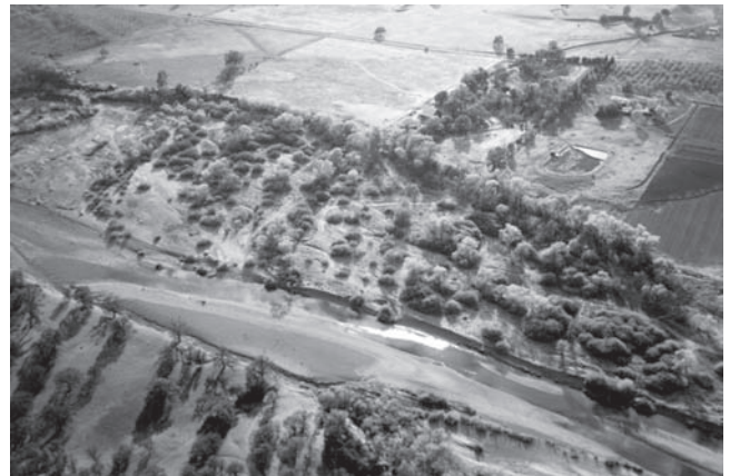
Fig. 1-5. Jacalitos Creek, California: the creek is attempting to outflank a highway bridge because the narrow bridge constriction and approach embankment prevent natural down-valley migration of meanders. Flow is from right to left. Photograph by V. J. Galay.
