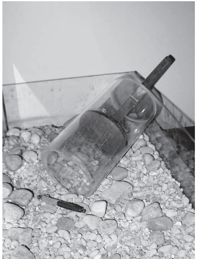
Fig. 5-3. The device used to collect areal samples. A thin layer of clay has been applied on the flat plate inside the piston.
