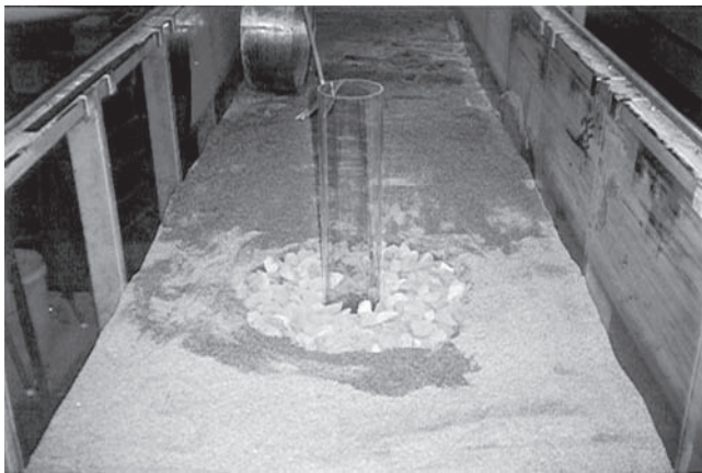
Fig. 11-6. Riprap protection at a model-scale bridge pier prior to testing (after Lauchlan 1999).
