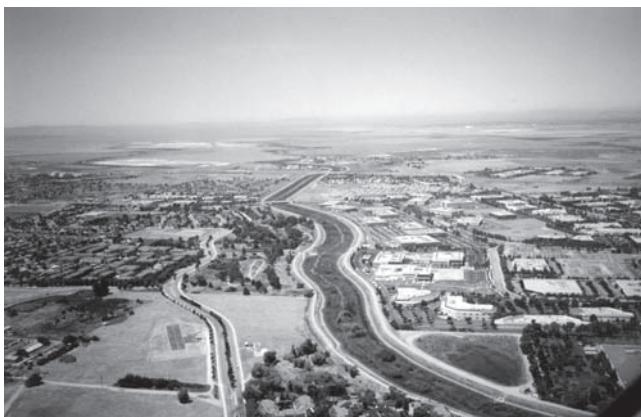
Fig. 1-6. Lower Guadalupe River below the City of San Jose, California: an example of a channelized urban river. The formerly meandering river was significantly straightened and leveed, restricting floodwaters to the main river channel. Formerly an agricultural area, the floodplain is now mainly occupied by urban and industrial development. View downstream. Photograph by R. C. MacArthur.
