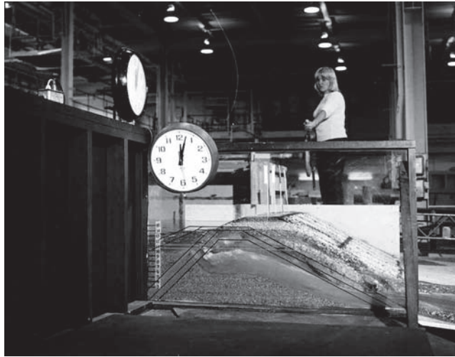
Fig. C-9. Fuse plug model test at Reclamation's hydraulic laboratory; pilot channel breach.
