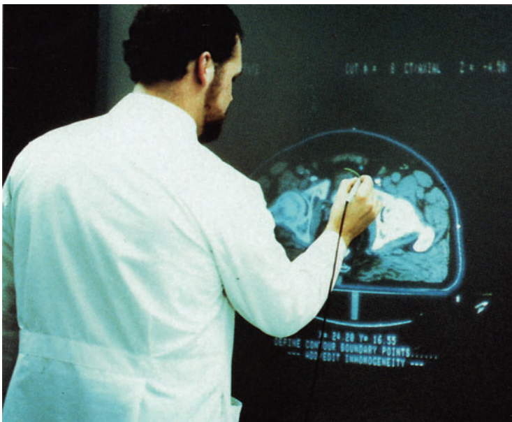
Fig. 23. The back-projection TV system for rapid entry of anatomic structures using CT scans (see p. 74)
