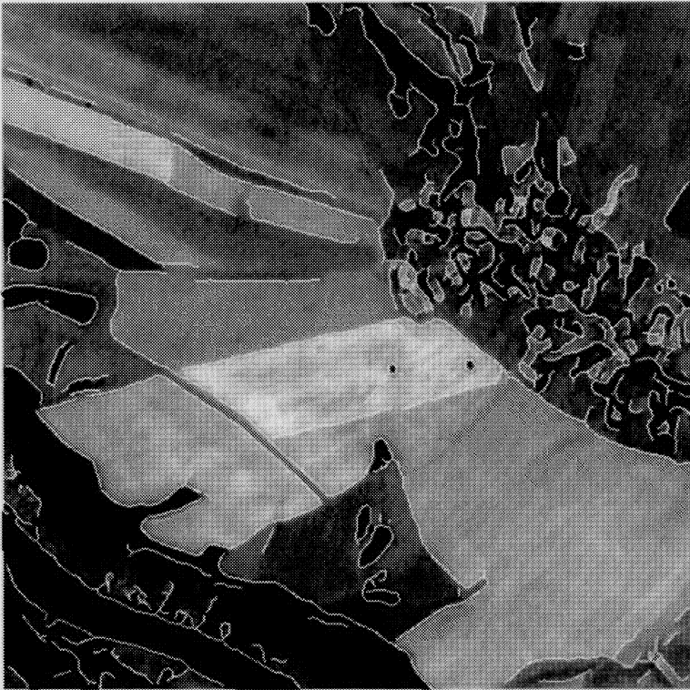
Figure 6.3-5: Extraction of linear features from IRS-1C panchromatic data (Data source: ANTRIX, SIE, Euromap Neustrelitz)
