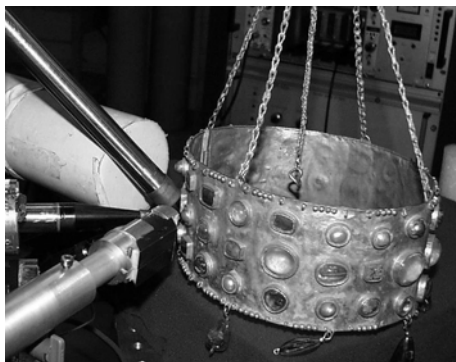
Figure II-2-4. Royal votive crown inlaid with gems positioned in front of the external beam set-up. Note the two Si(Li) detectors and HPGe in the back.
