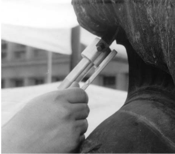
Fig. I-2-16. In-situ examination of the patina surface of the outdoors bronze monument Th Kolokotronis using PXRF-C2 portable spectrometer.
