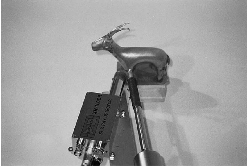
Fig. I-2-11. In-situ EDXRF analysis at the Akrotiri archaeological site in Thera of the gold ibex figurine using PXRF-B portable spectrometer.
