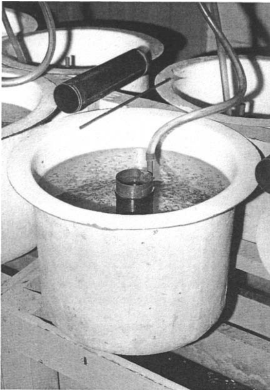
FIGURE 2 Planktonkreisel for rearing lobster larvae (so-called "Hughes' pot") developed at the Massachusetts State Lobster Hatchery and Research Station on Martha's Vineyard. (Courtesy of J. R. Factor.)
