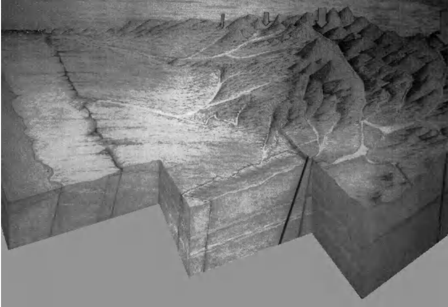
Figure 24. Perspective illustration of the megawatershed model applied in the Red Sea province of Sudan. Arrows illustrate mountain recharge to fracture systems and alluvial storage. (See color insert.)
