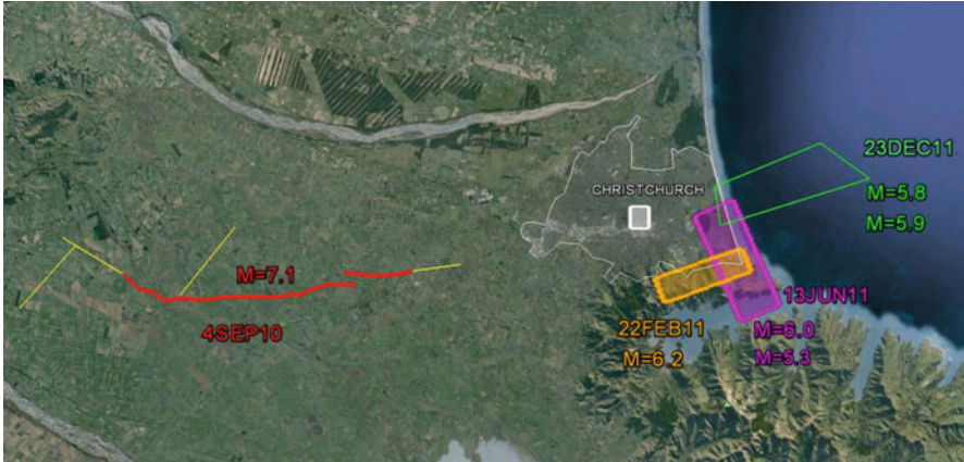
Fig. 1.2 Causative faults of the 2010–2011 Christchurch earthquakes (4 September 2010 earthquake, red line = trace of surface rupture, yellow lines = subsurface rupture; 22 February 2011 earthquake, orange area = fault area projection; 13 June 2011 earthquakes, magenta area = fault area projection; 23 December 2011 earthquake, green line = general source area); the Central Business District (CBD) of Christchurch is shown with the white square
