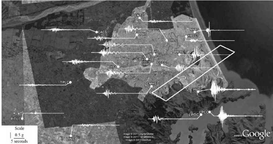
Fig. 1.3 Observed fault-normal horizontal acceleration time series at various locations in the Christchurch region from the 22 February earthquake
