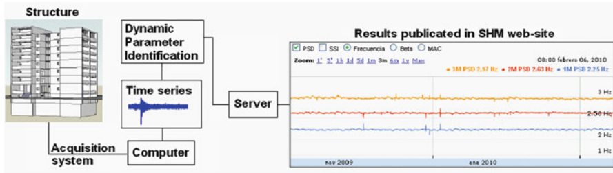
Fig. 8.6 Structural health monitoring network workflow
