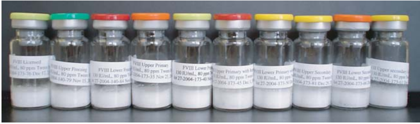
Figure 32.5. Photo of lyophilized product for all 10 cycles. Pictured from left to right: process set point, upper freezing, lower freezing, upper primary, lower primary, upper primary with increased ramping rate, lower primary with decreased ramping rate, upper secondary, lower secondary, and upper secondary with increased ramping rate.
