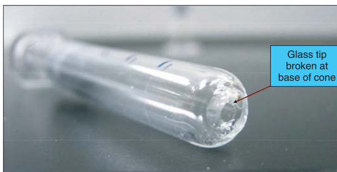
Figure 36.8. A 1-mL-long syringe barrel after breaking off the tip at the shoulder. The resulting hole in the barrel is large enough that product fluid flow resistance is no longer a factor when measuring glide force.
