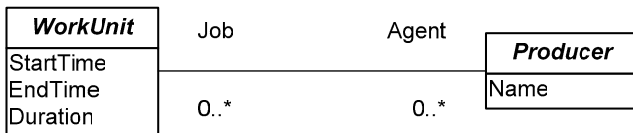
Fig. 4.11. Connection between the process (Work Unit) and people (Producer) sides of the metamodel
