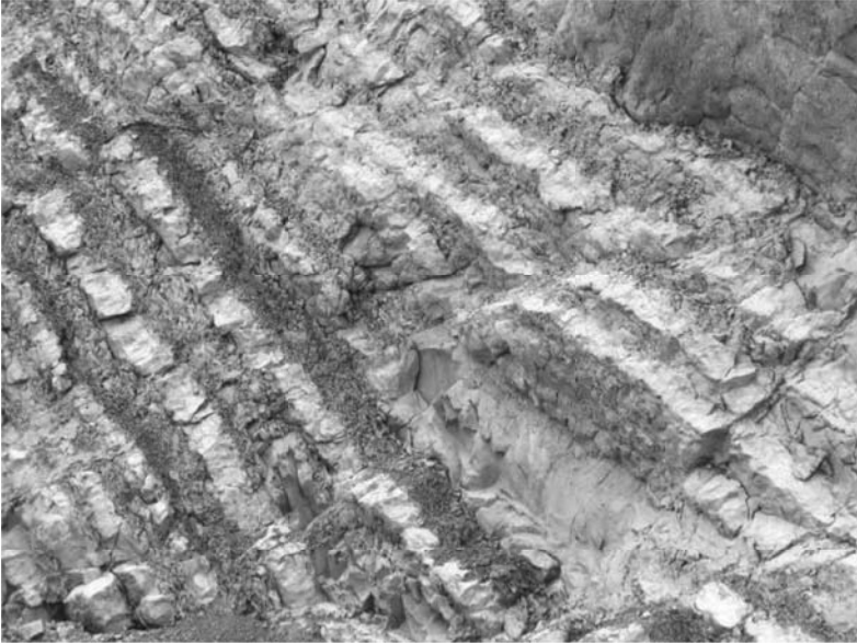
Figure 4.5 Anisotropy in chalk strata composed of alternating hard and soft layers (dimension across the picture diagonal \sim 3 m, Lower chalk, Isle of Wight, UK).
