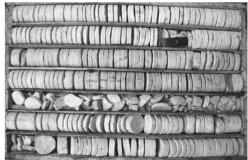
'Exposure' 6. Marble drillcore from the Jinping II tunnelling site, China
