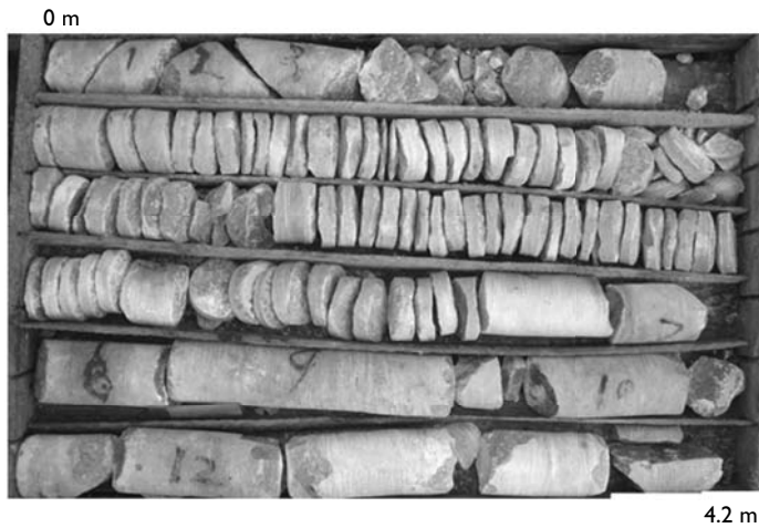
Figure 6.50 Rock discing in the rock surrounding access tunnel A at overburden 2430 m.
