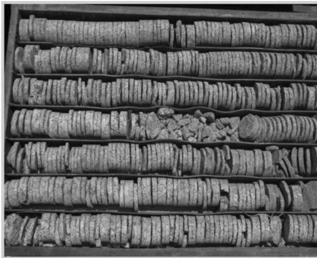
Figure 6.9 Extreme rock core discing caused by high in situ rock stress and the process of core drilling (from Feng & Hudson, 2011).
