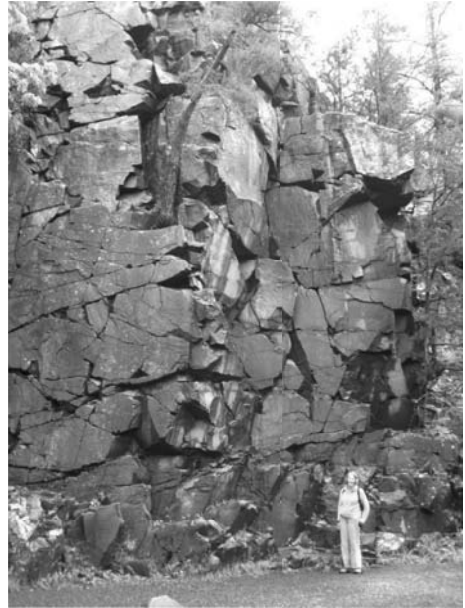
Exposure 2. Shattered basaltic rock mass, Minnesota, USA
