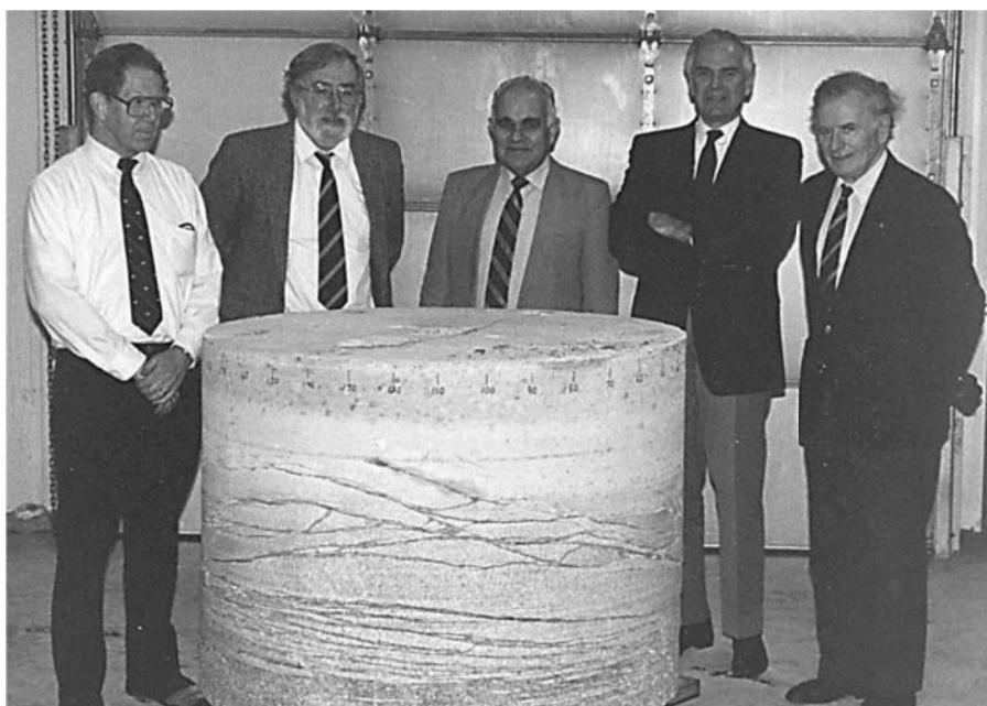
Figure 5.17 'Discing' of a large rock core due to the effect of the in situ stress when coring takes place. Left to right: Neville Cook, John Hudson, Evert Hoek, Norbert Morgenstern, Charles Fairhurst in 1991.
