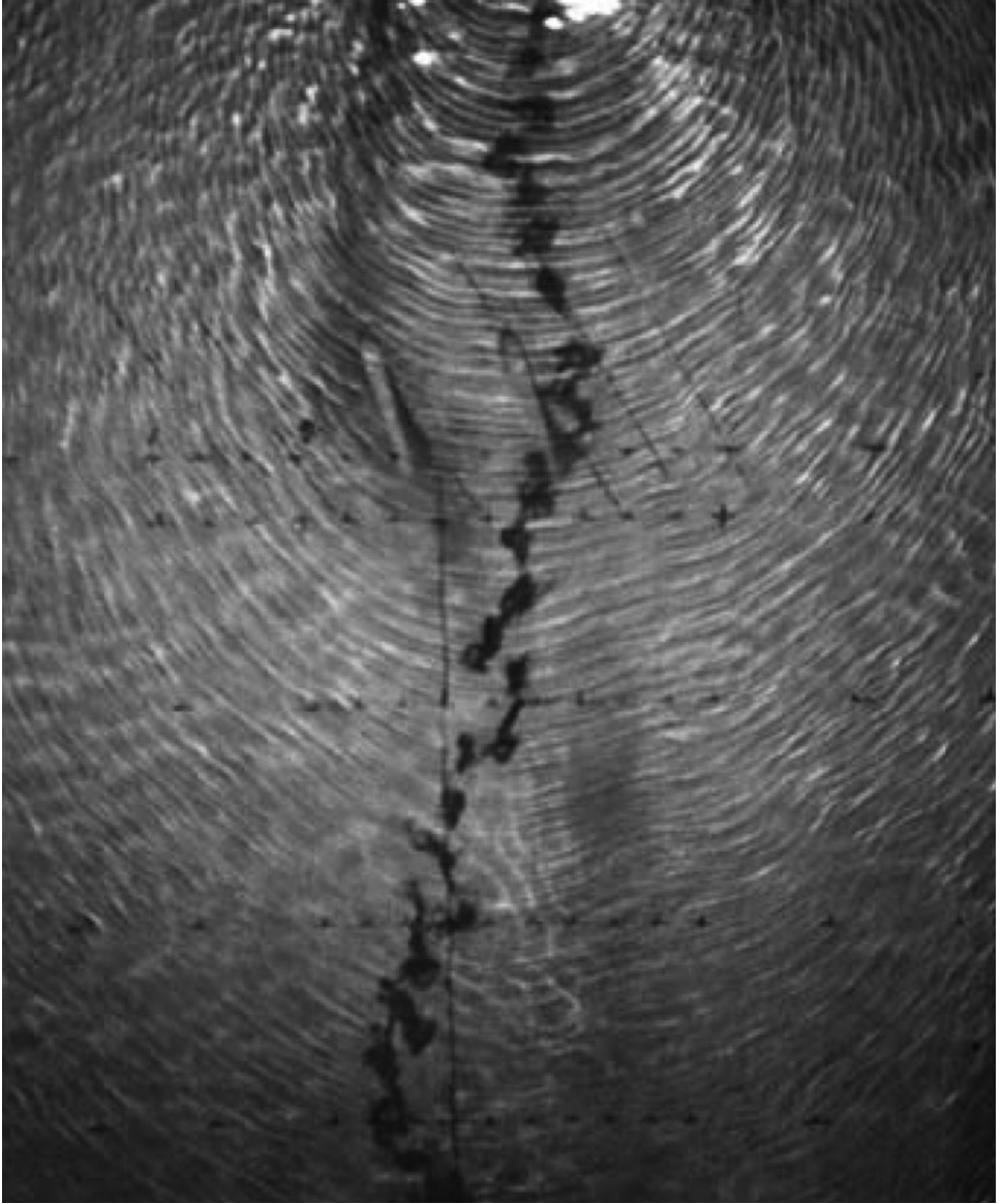
Figure 1-9. Top view of vane pair with water flowing (from top of photo to bottom) at depth about twice the vane height; dye injected upstream (blue at the bottom and red at the surface) shows vane-induced circulation.
