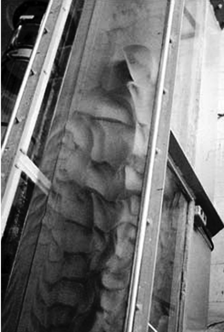
Figure 1-11. Vane in sand-bed channel deflecting sediment to one side of the channel.
