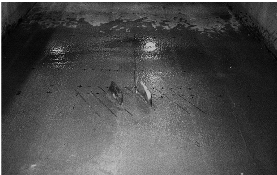
Figure 1-8. Two vanes at centerline of open channel. View is downstream before water is admitted.
