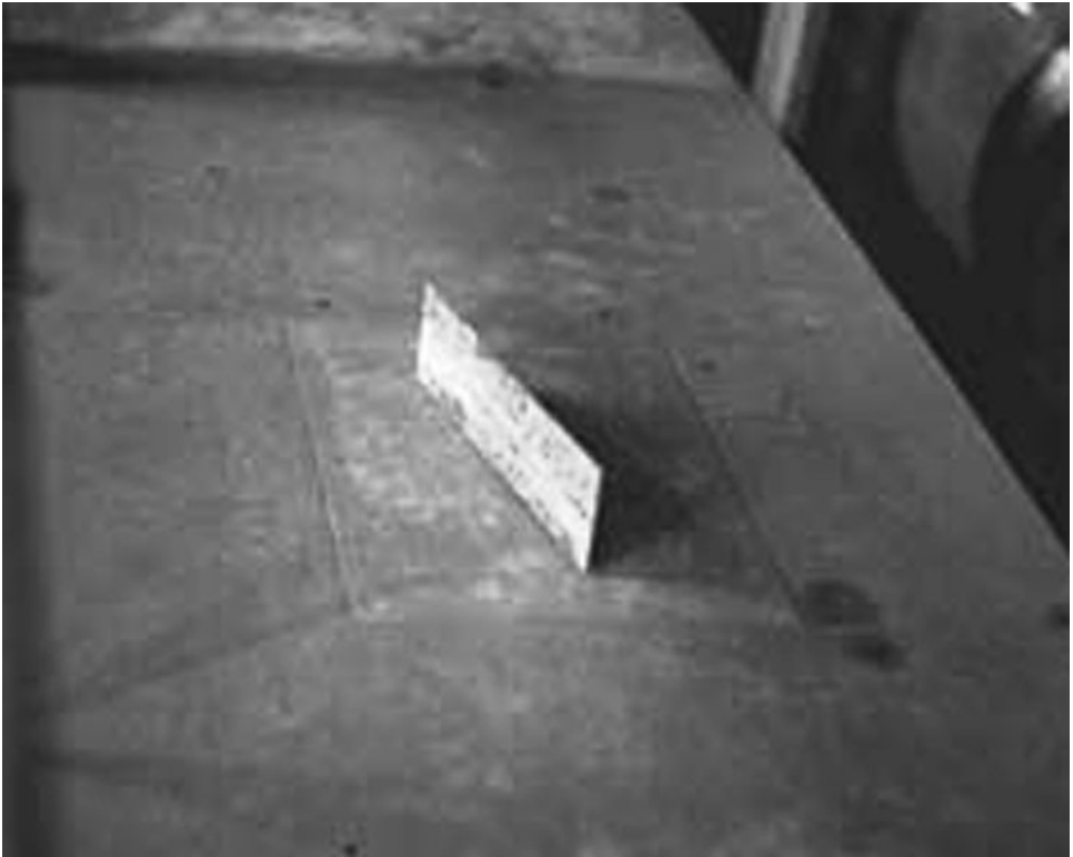
Figure 1-16. Lift and drag measurements on vane profiles in laboratory flume resulted in improved vane design.
