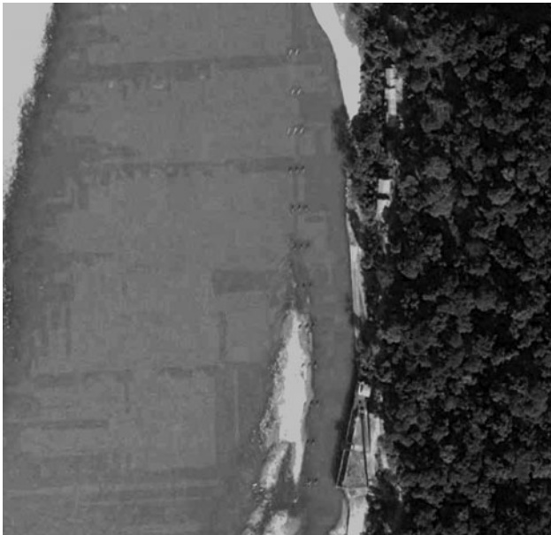
Figure 5-66. 2004 DigitalGlobe image showing low flow in Kosi River near the intake. The image shows the vane system and intake. Flow is from top of image. The vane system is seen to maintain a near-bank channel toward the intake. The vane-induced sand deposit on the far side of the vane system is also clearly visible. Courtesy of DigitalGlobe.
