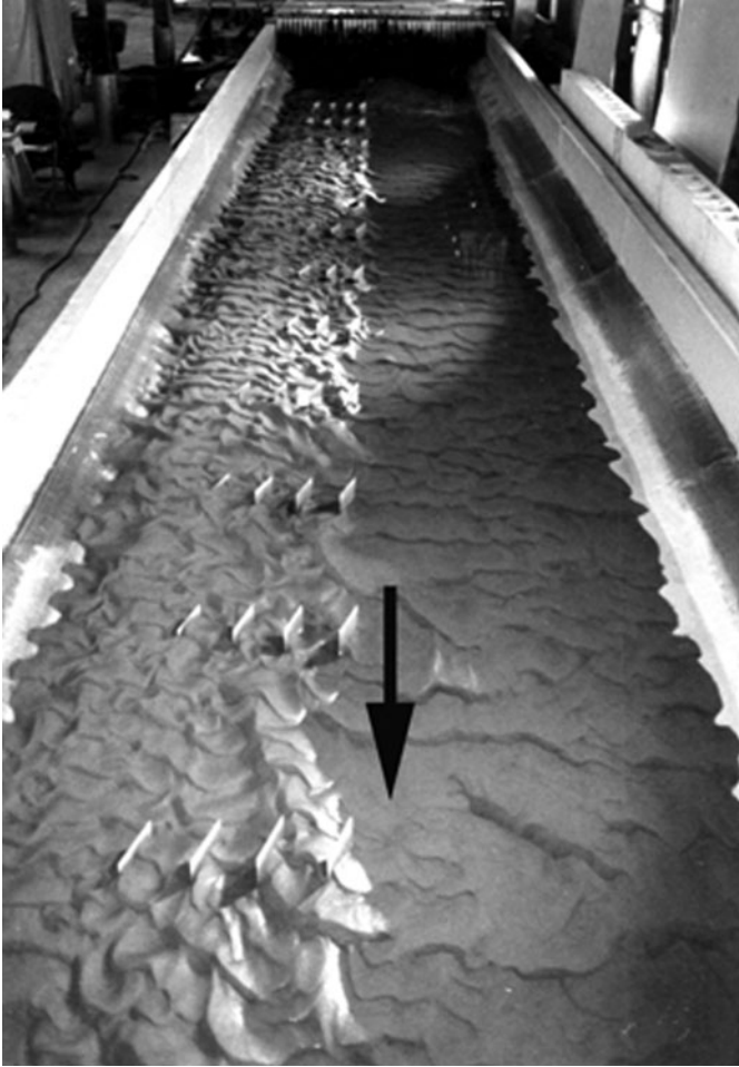
Figure 3-11. Upstream view of nearly drained, straight channel with vanes. Source: Odgaard and Wang (1991), ASCE.
