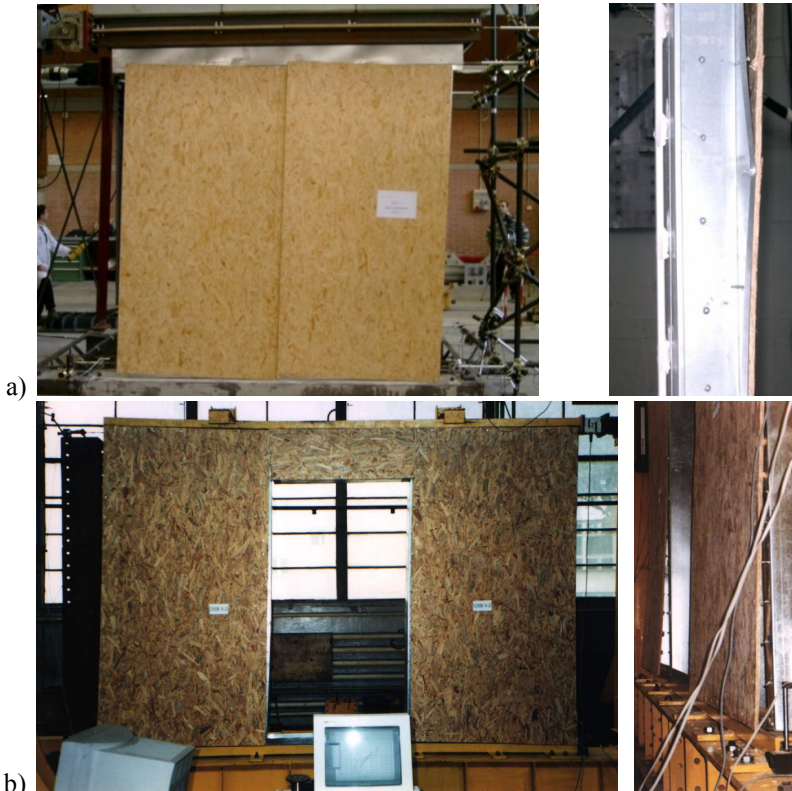
Figure 8.49 – Global collapse mechanism of a wall due to failure of sheathing to frame connections
