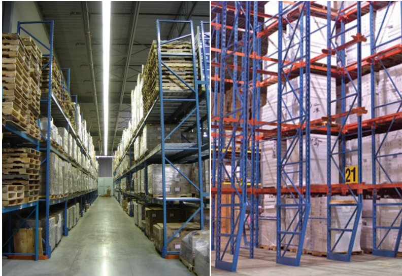
Figure 1.35 – Storage rack systems ( http://en.wikipedia.org/wiki/Pallet_racking )
