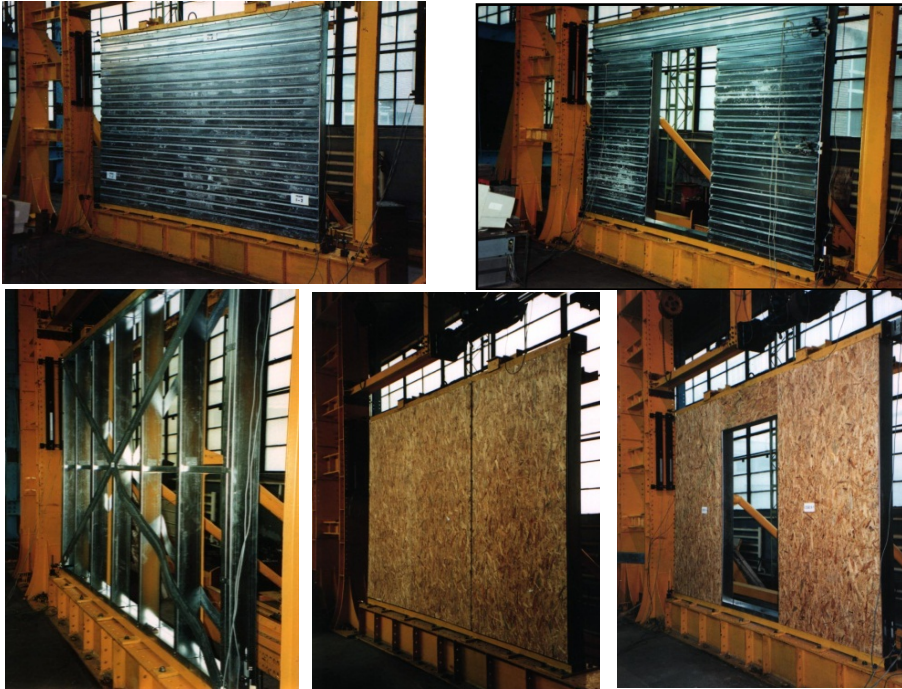
Figure 8.51 – Typical shear tests of a wall (Fülöp & Dubina, 2004a)
