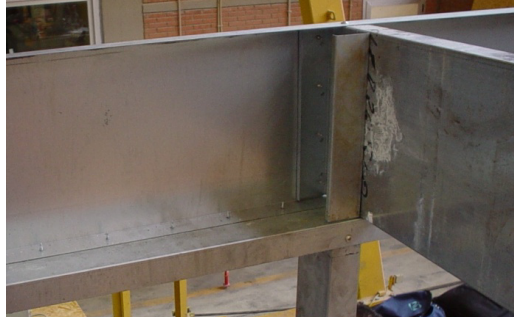
Figure 8.37 – “Web stiffener” profile
