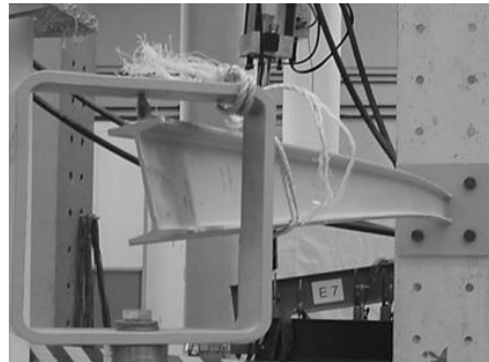
a) LT buckling of a slender cantilever beam (SSEDTA, Lecture 12) b) LT buckling of a slender cantilever beam in testing (da Silva et al , 2010)
