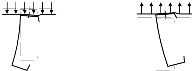
a) Sheathing on flange in compression b) Sheathing on flange in tension Figure 8.41 – Stabilizing effect of sheathing on C-profile under bending
