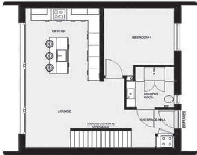
Ground floor plan showing two adjacent modules. (Courtesy of Futureform.)
