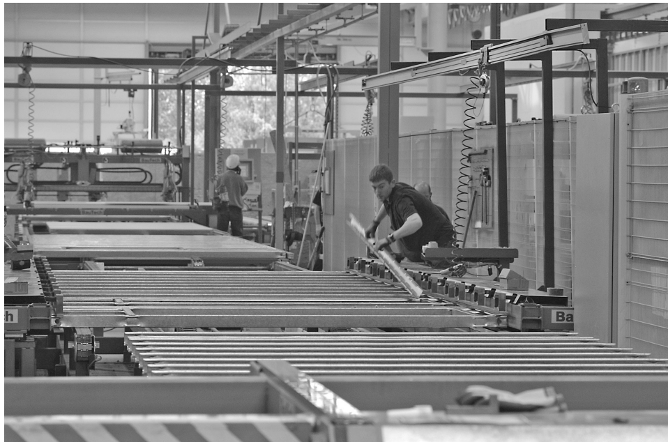
Figure 17.3 Assembly of light steel panels in production. (Courtesy of Unite Modular Solutions.)
