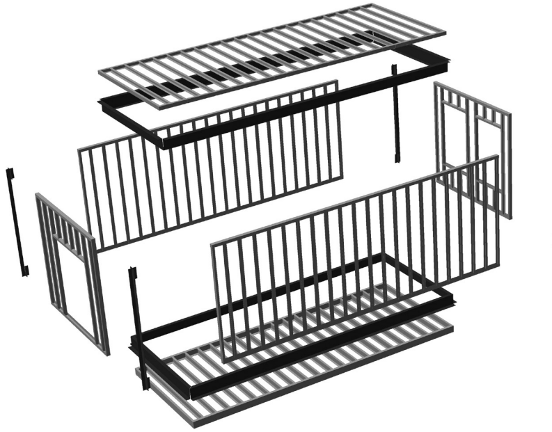
Figure 2.3 Assembly of a module from five panels, corner posts, and a floor cassette.
