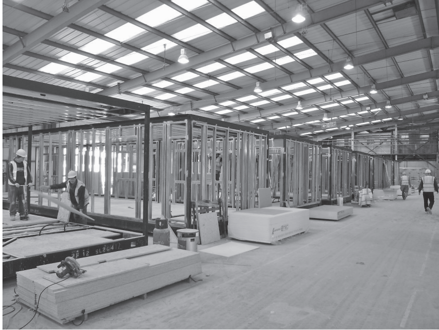
Figure 17.2 Static production of modular units. (Courtesy of Caledonian Modular.)
