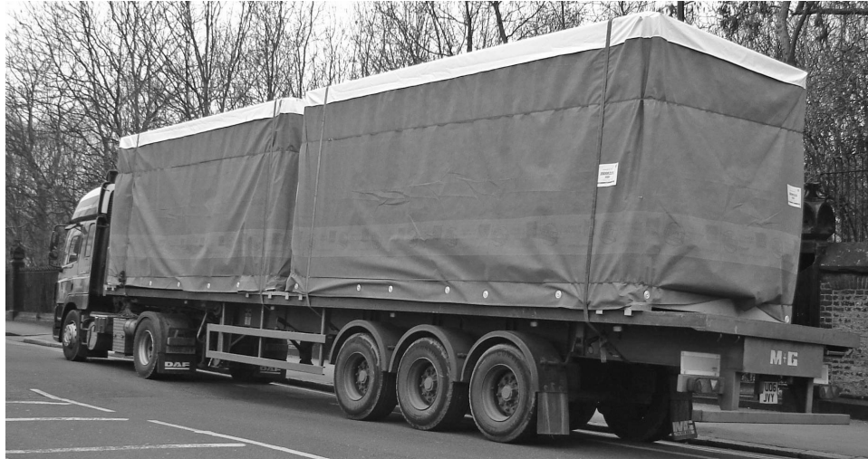
Figure 16.12 Delivery of two modules on a lorry. (Courtesy of Unite Modular Solutions.)
