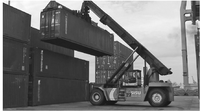
Figure 4.6 Lifting of shipping containers from their corners. (Courtesy of Matthias Hamm.)
