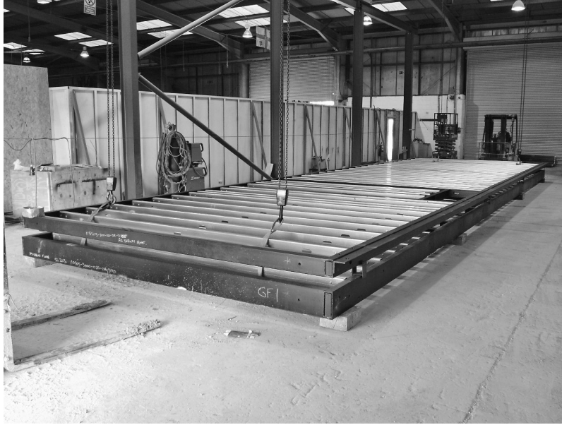
Figure 17.1 Pre-manufacture of steel floor and ceilings in hot-rolled steel and light steel elements. (Courtesy of Caledonian Modular.)
