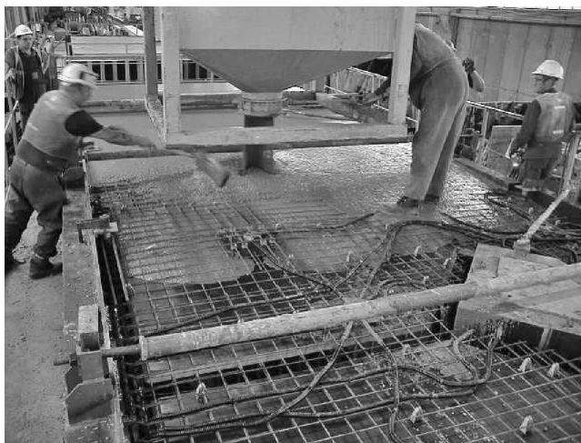
Figure 17.9 Casting a modular unit from the top using self-compacting concrete. (Courtesy of Tarmac Precast Ltd.)
