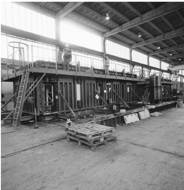
Figure 3.7 Casting a modular concrete unit. (Courtesy of Tarmac Precast Ltd.)
