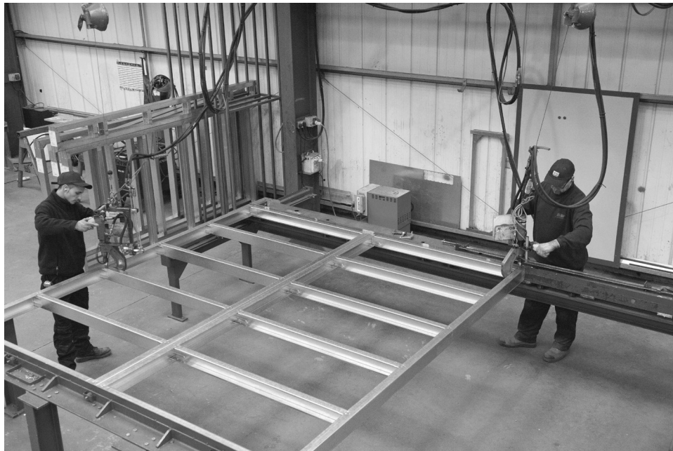
Figure 1.22 Manufacture of light steel wall panel. (Courtesy of BW Industries.)
