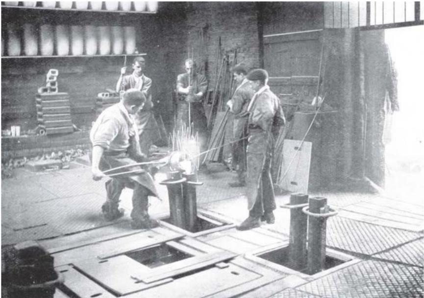
**Figure 3.** Men teeming crucible steel at Jessops' Brightside Steel Works, Sheffield. c. 1911.
