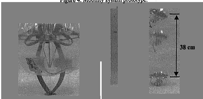
Figure 5. Autonomous Microbot prototype performing hops of 38 cm.
