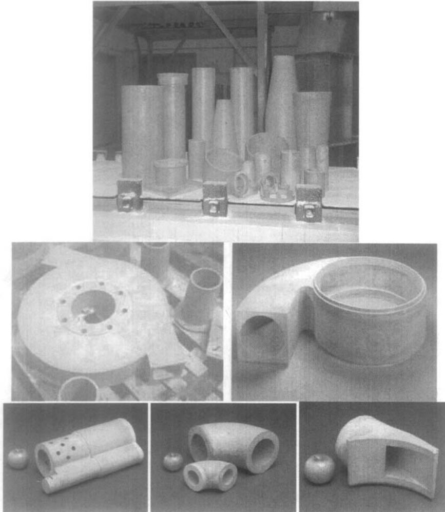
Fig. 7. Different SiC-based ceramic products manufactured through thixotropic casting
