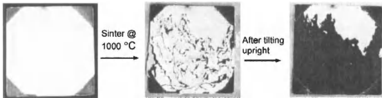
Figure 6: Example of how Haynes 230 samples behaved when exposed to temperatures over 600 °C. For each case, this behavior was typical and is believed to be due to the lack of a bond coat, which helps alleviate the coefficient of thermal expansion mismatch.
