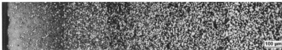
Figure 4. Optical microscopy image of sintered sample with S3 slip, light phase: NiCr8020, dark phase: TZ-8YS, left side: upper surface
