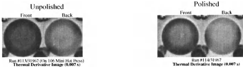
Figure 7. Results from pulsed thermography for the less polished pair of joined substrates (left) and for the more polished pair (right).
