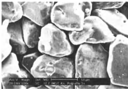
Figure 11. Completely sintered specimen with 70 \mu\text{m} coarse particle size but with hardly any neck formation.
