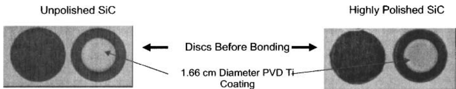
Figure 2. Photos of the coated and uncoated sets of SiC discs before bonding. The less polished discs are on the left and the more polished discs are on the right.
