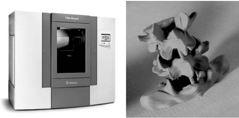
Figure 1.2 Maxum machine, along with a spine model made using FDM (courtesy of Stratasys)
