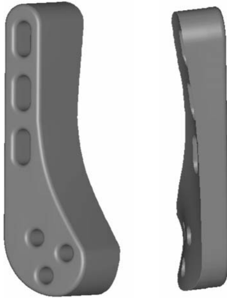
Figure 9.4 CAD model of the custom-designed bone plate, showing the front and the backside
