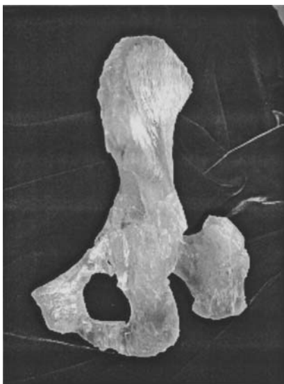
Figure 2.4 SLA model of the bone of a hemipelvis, produced using CT images (courtesy of Medical Modeling LLC)
