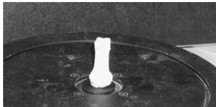
Figure 7.9 Rotary stage set with bone sample on the centre
