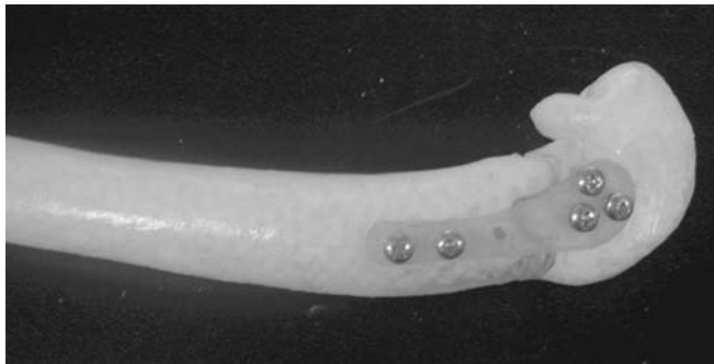
Figure 9.5 SLA model of the fractured distal femur and the custom-designed bone plate
