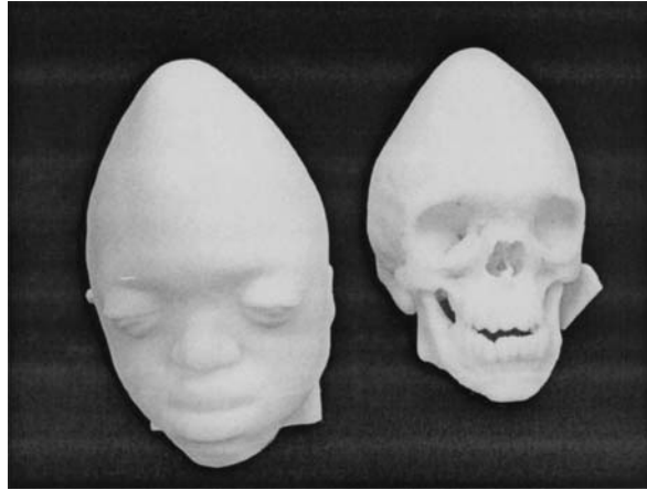
Figure 2.6 Two-color stereolithography model showing a myxoma tumor of the right temporomandibular Joint (courtesy of MedicalModeling LLC)
