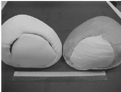
Figure 4.5 RP models fabricated by FDM (left) and SLA systems
