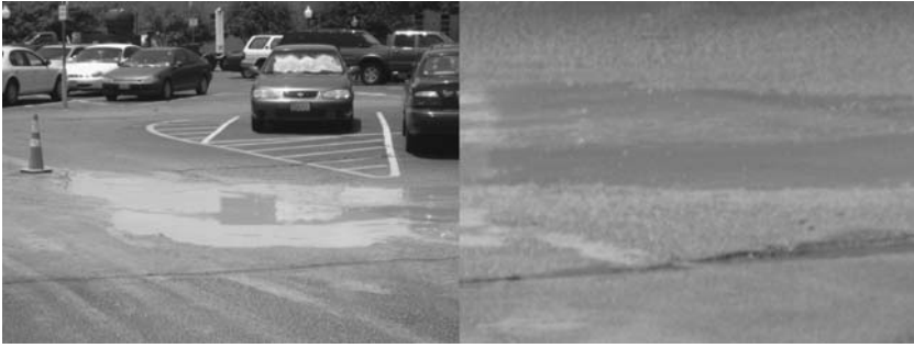
FIGURE 5.10 Inadvertent fluid returns in the urban environment.
