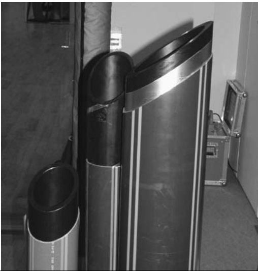
FIGURE 6.19 Protecting the HDPE pipe from shards. (Source: Handbook of Polyethylene Pipe , 2008.)
