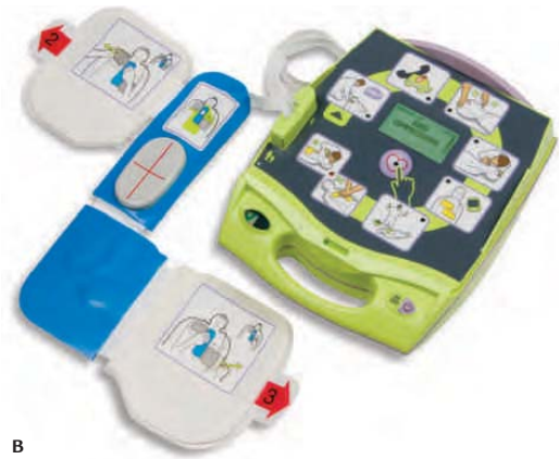
Figure 33.22 Automatic external defibrillators. A Signs in public places indicate where AEDs are available. B An AED is designed to be used by nonmedical personnel. Voice commands and pictures instruct the user in how and where to place the electric paddles. The device then assesses the need for defibrillation and, if necessary, delivers an electric shock.
